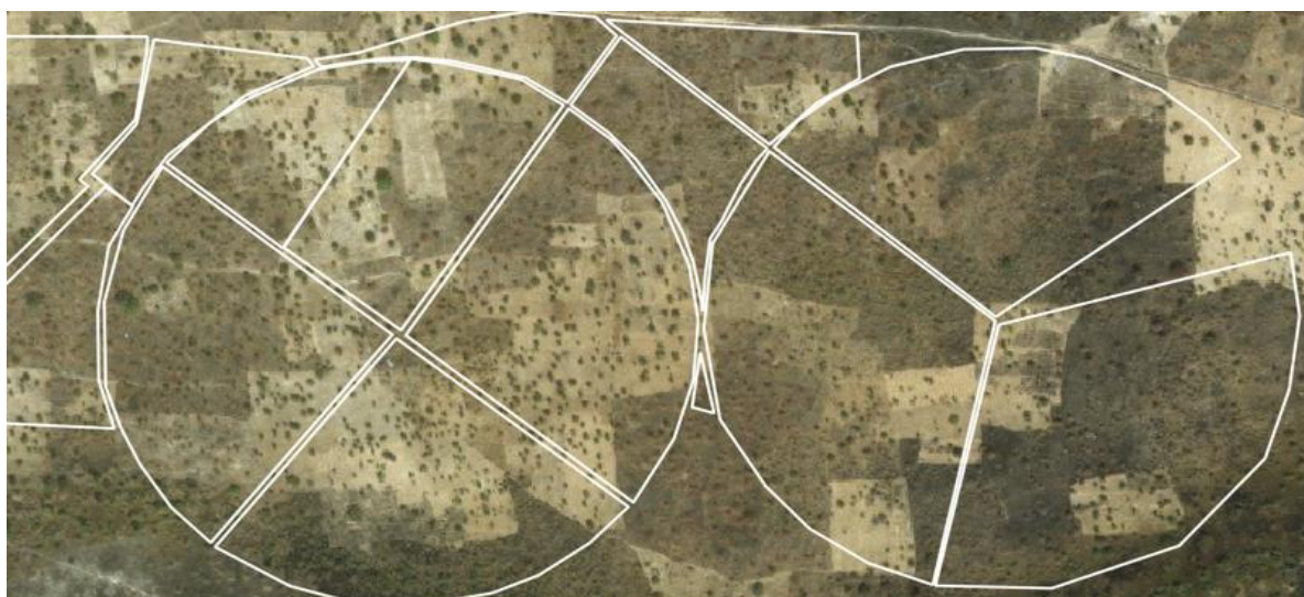
Figure 1. An example of potential training data error that can arise when image interpretation is conducted on older imagery. The underlying imagery is from Bing Maps, which shows smallholder agricultural fields near Kulpawn, Ghana. The white polygons were collected by a team of mappers (hired by Meridia) on the ground using handheld GPS in 2018. The smallholder fields were replaced by larger center-pivot irrigation fields sometime after the imagery in the base map was collected.
