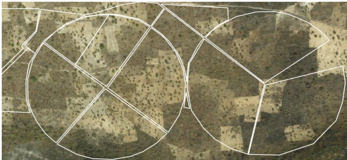
Figure 1. An example of potential training data error that can arise when image interpretation is conducted on older imagery. The underlying imagery is from Bing maps, which shows smallholder agricultural fields near Kulpawn, Ghana. The white polygons were collected by a team of mappers (hired by Meridia) on the ground using handheld GPS in 2018. The smallholder fields were replaced by larger center-pivot irrigation fields sometime after the imagery in the base map was collected.
