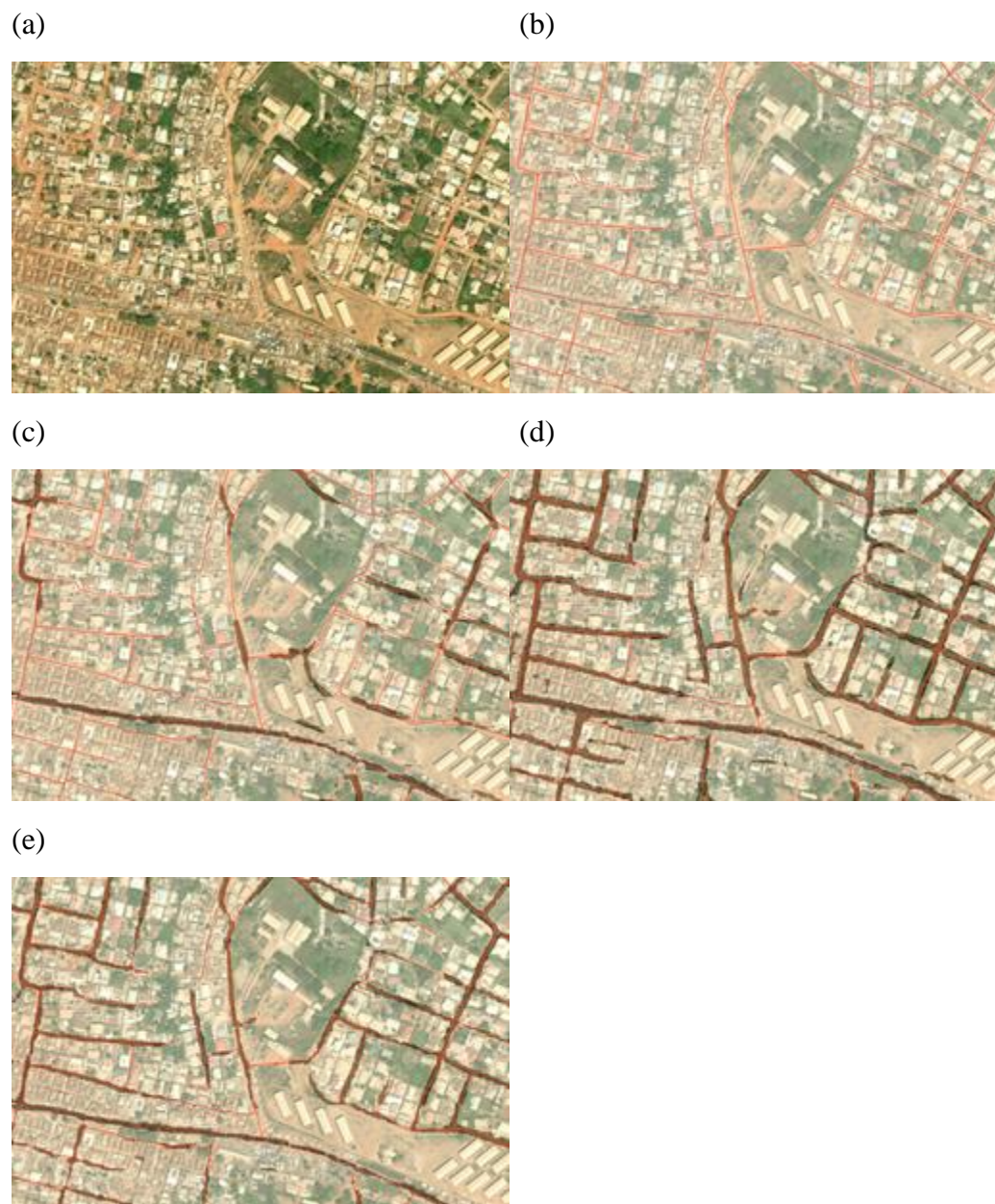
Figure A2: Sample prediction results in Kumasi, Ghana. (a) Input imagery. (b) Predictions from the Las Vegas model. (c) Predictions from the Khartoum model. (d) Prediction from the Kumasi model. (e) Predictions from the Khartoum Model retrained in Kumasi. [in panel b-e model predictions are in shaded color overlaid with validation labels in red on top of imagery]
