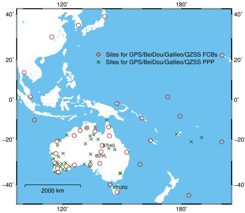
**Fig. 1** Distribution of multi-GNSS stations from days 335 to 365 in 2017. 35 stations denoted as red open circles are used to estimate FCB products for GPS, BeiDou, Galileo and QZSS satellites, while 41 stations denoted as green crosses contribute to GPS/BeiDou/Galileo/QZSS kinematic PPP. Three stations BDVL, BUR2 and STHG are especially denoted.
