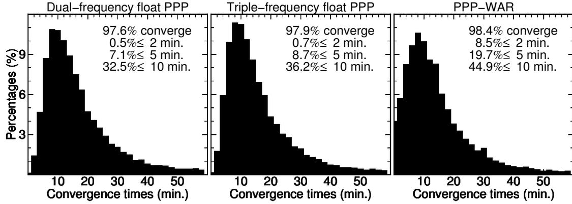
**Fig. 5** Distribution of convergence times (minutes) of three types of solutions for all stations on all days. The solutions include dual- and triple-frequency float PPP and PPP-WAR. The percentages for those solutions converging successfully within 2, 5 and 10 minutes are plotted at the top right corner of each panel.
