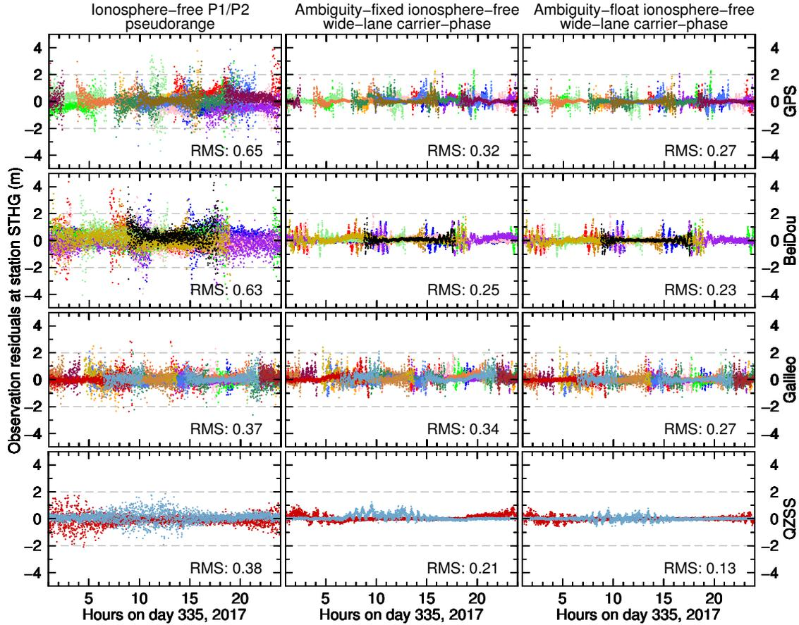
**Fig. 4** GPS, BeiDou and Galileo observation residuals (m) at station STHG on day 335, 2017. Three types of residuals are shown for ionosphere-free P1-P2 pseudorange from dual-frequency float PPP, ambiguity-fixed and ambiguity-float ionosphere-free wide-lane carrier-phase from triple-frequency PPP (see Eq. 14). All residuals are computed by fixing station coordinates, and color coded against satellites. The mean RMS of residuals (m) are plotted at the bottom right corner of each panel.
