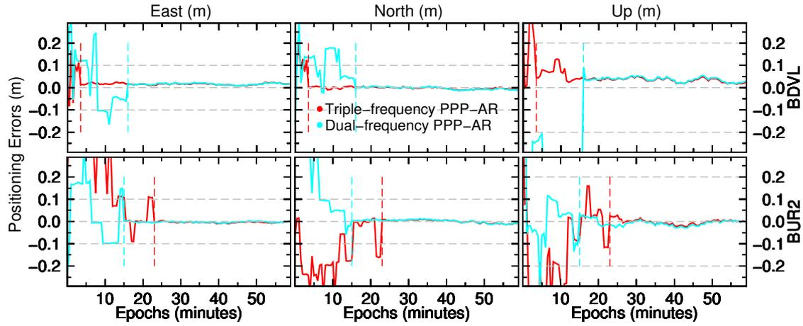
**Fig. 6** Positioning errors (m) for east, north and up components at stations BDVL and BUR2. Two solutions, i.e., dual- and triple-frequency PPP-AR, are presented. The vertical dashed red and cyan lines mark the epochs when successful PPP-AR is achieved. Note that triple-frequency PPP-AR is augmented by PPP-WAR discussed in section 4.2.
