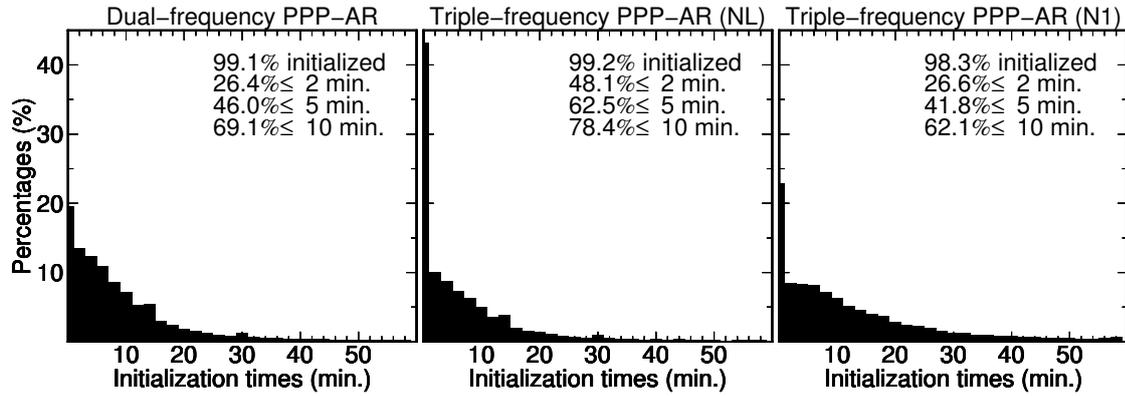
**Fig. 7** Distribution of initialization times (minutes) for dual- and triple-frequency PPP-AR at all stations on all days. The percentages of the initialization times that are shorter than 2, 5 and 10 minutes are plotted at the top right corner of each panel. Note that triple-frequency PPP-AR with N1 ambiguities fixed is shown in the rightmost panel.
