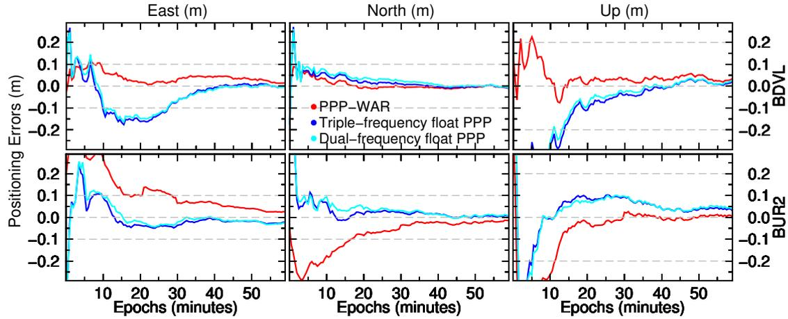
**Fig. 3** Positioning errors (m) for the east, north and up components at stations BDVL and BUR2 for PPP-WAR and ambiguity-float solutions. PPP-WAR indicates that both extra-wide-lane and wide-lane ambiguity fixing have been accomplished.
