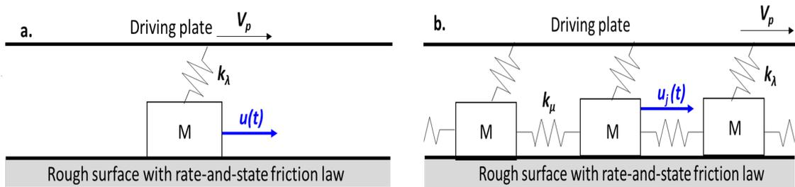
**Figure 1:** Schematic representation of the Burridge Knopoff models coupled with the rate-and-state friction law (a) single degree of freedom slider block coupled by a spring loader plate representing the other side of the fault. (b) spring connected chain of blocks, elastically coupled to a driver plate moving a constant velocity  $V_p$ . The surface upon which the blocks slip is rough and the friction force holding the slider in place is governed by a rate-state friction law.
