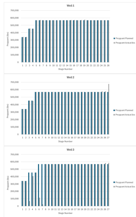
Fig. 7 Design vs. actual proppant placed for each stage across a three-well pad completed with a plug-and-perforate stimulation treatment design. The designed proppant volumes were pumped on 95% of the stages.
