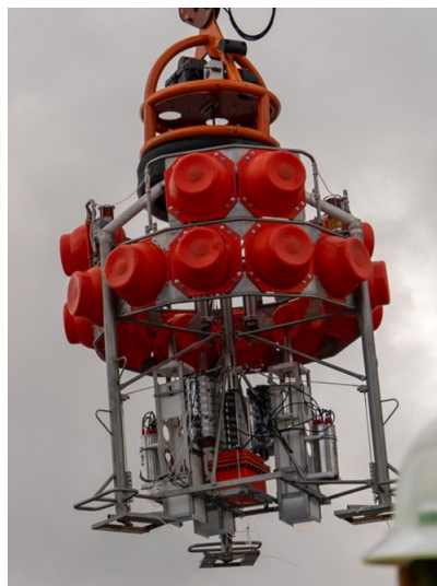
Supplementary Fig 4: Image of the benthic chamber lander recovery after the closed-bottom chamber experiment (AKS287). Note that all three chamber bottom lids (doors) are closed. The original image has been cropped.
