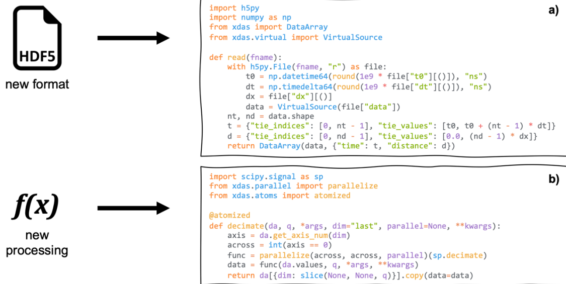
Figure 6. Extensibility of Xdas. (a) Adding the support for a new file format generally consists into providing the path to the data array, and parsing the start time and spatial and temporal spacing. Here a hypothetical simple file format is used as example. For real world application, the four lines into the with statement block must be adapted. (b) Wrapping a signal processing function that is applied along one axis require to convert the dimension name in its related axis number, processing the data (optionally in a parallelized manner), and handling coordinates changes if any. Here we reimplement the decimate function almost as it is implemented in Xdas.
