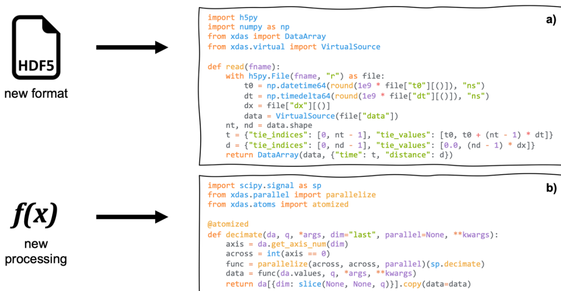
Figure 6. Extensibility of Xdas. (a) Adding the support for a new file format generally consists into providing the path to the data array and parsing the start time and spatial and temporal spacing. Here a hypothetical simple file format is used as example. For real world application, the four lines into the with statement block must be adapted. (b) Wrapping a signal processing function that is applied along one axis require to convert the dimension name in its related axis number, processing the data (optionally in a parallelized manner), and handling coordinates changes if any. Here we reimplement the decimate function almost as it is implemented in Xdas.
