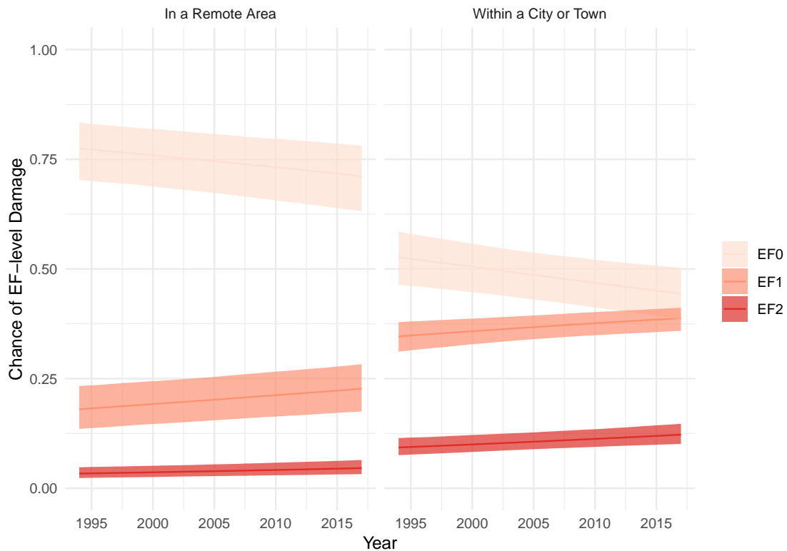
369 FIG. 7. Marginal trends in the distribution of EF rating (EF0, EF1, and EF2). Trends are estimated by setting 370 the distance to 135 km for remote areas and 0 km for inside a city or town.
