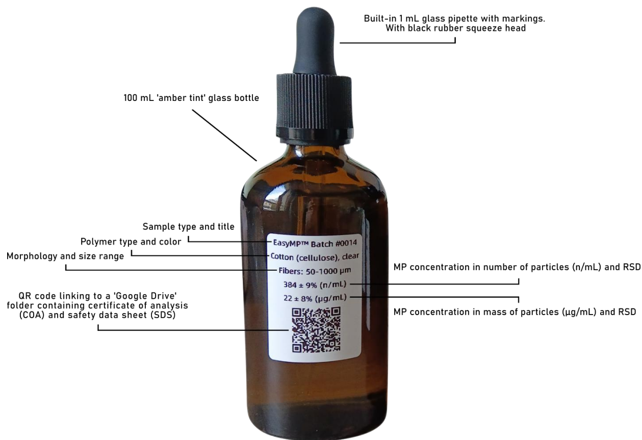
94 95 Figure 2 - 100 mL EasyMP™ 'Fiber sample #1', containing cotton (cellulose) fibers from 50-1000 \mu\text{m} in length. The label provides 96 basic information such as particle concentration in both counts (n/mL) and mass ( \mu\text{g/mL} ). The QR code grants access to a dedicated 97 cloud folder containing the COA and SDS.
