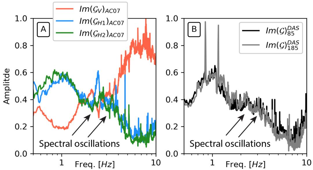
**Fig. 2. Single component Green's functions for DAS and velocimeter.** (A)  $Im(\mathcal{G}_{ii})$  computed from the tri-axial AC07 velocimeter and; (B) computed for the two orthogonal channels 85 and 185.
