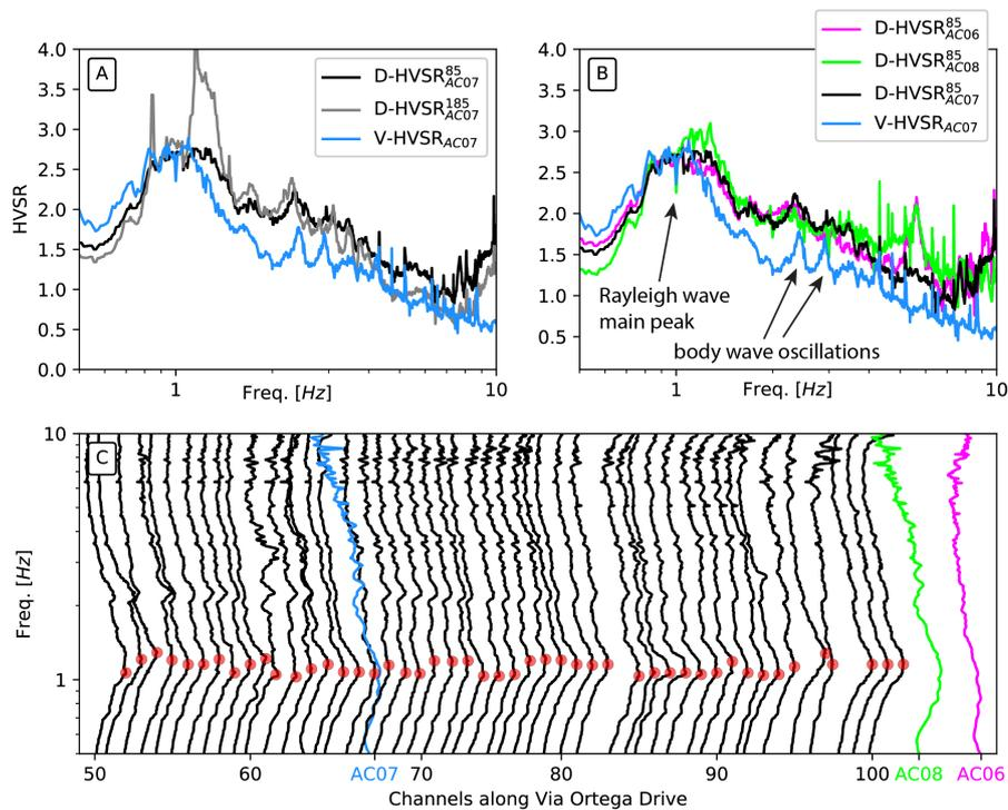
**Fig. 3. Comparison between DAS and velocimeter H/V spectral ratios.** (A) D-HVSR computed with channel 85 and 185 and V-HVSR for station AC07. (B) Comparison between the V-HVSR at station AC07 and the D-HVSR at channel 85 computed with the vertical component of the three different velocimeters on campus. (C) All the D-HVSR computed along Via Ortega (black) along with the three V-HVSR (color). The frequency of the main D-HVSR peaks are highlighted by a red dot.
