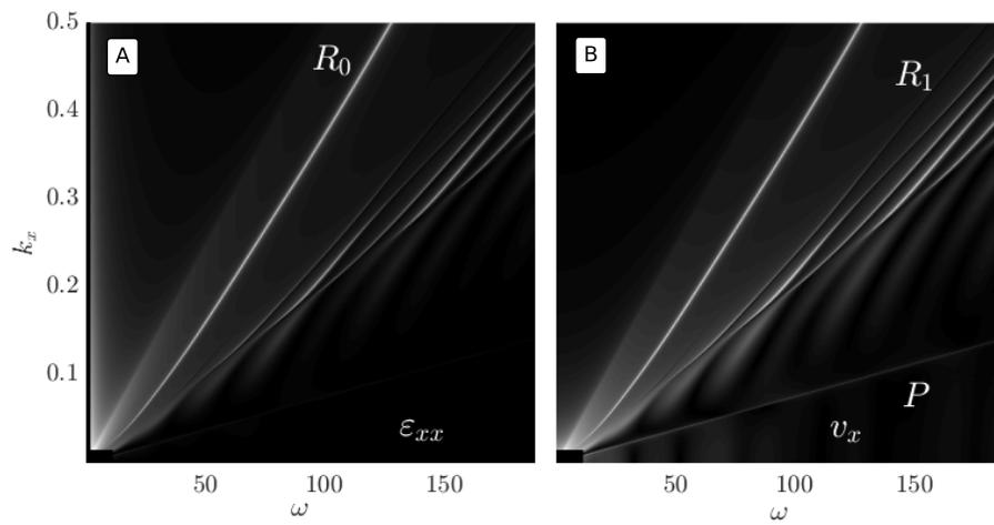
**Fig. S 4.**  $\omega - k_x$  diagrams for strain and velocity. (A) strain  $\omega - k_x$  diagram. (B) velocity  $\omega - k_x$  diagram. Both diagrams are obtained by simulating the wave propagation with the Discrete Wave Number method using velocity model shown in Fig. 2. The color scale is logarithmic and light colors correspond to higher energies.  $R_0$  and  $R_1$  indicate the fundamental and first higher mode of the Rayleigh wave, respectively.  $P$  is the  $P$ -wave.
