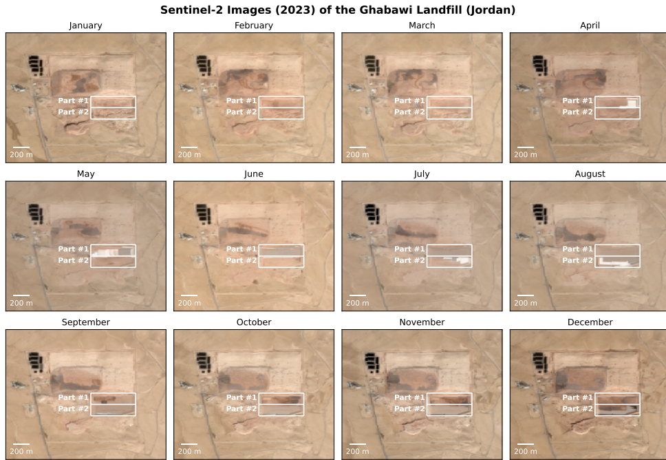
Fig. S17 Monthly Sentinel-2 RGB images [12] captured in 2023 showing the Ghabawi Landfill in Jordan. The two white rectangles highlight two cells within the recently developed southern section. Movie S1 shows a time-lapse sequence of all cloud-free Sentinel-2 RGB images captured throughout 2023.
