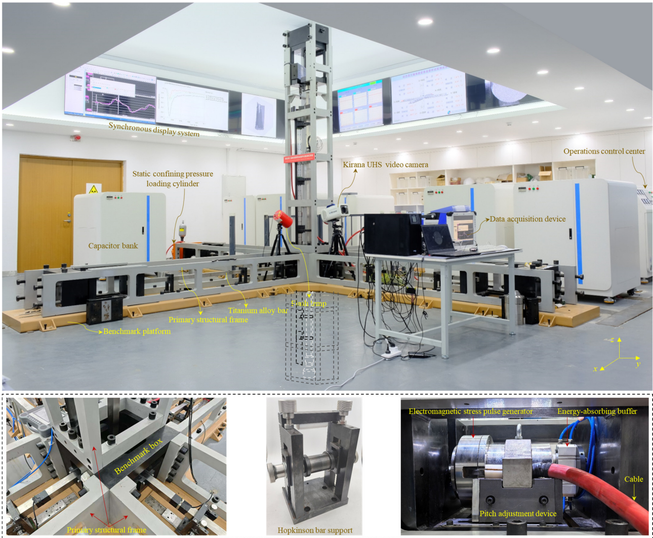
Fig. 1 Dynamic true triaxial electromagnetic Hopkinson bar (DTEHB) system: (a) Overall system configuration; (b) Three key components of the 3D centering and leveling system
