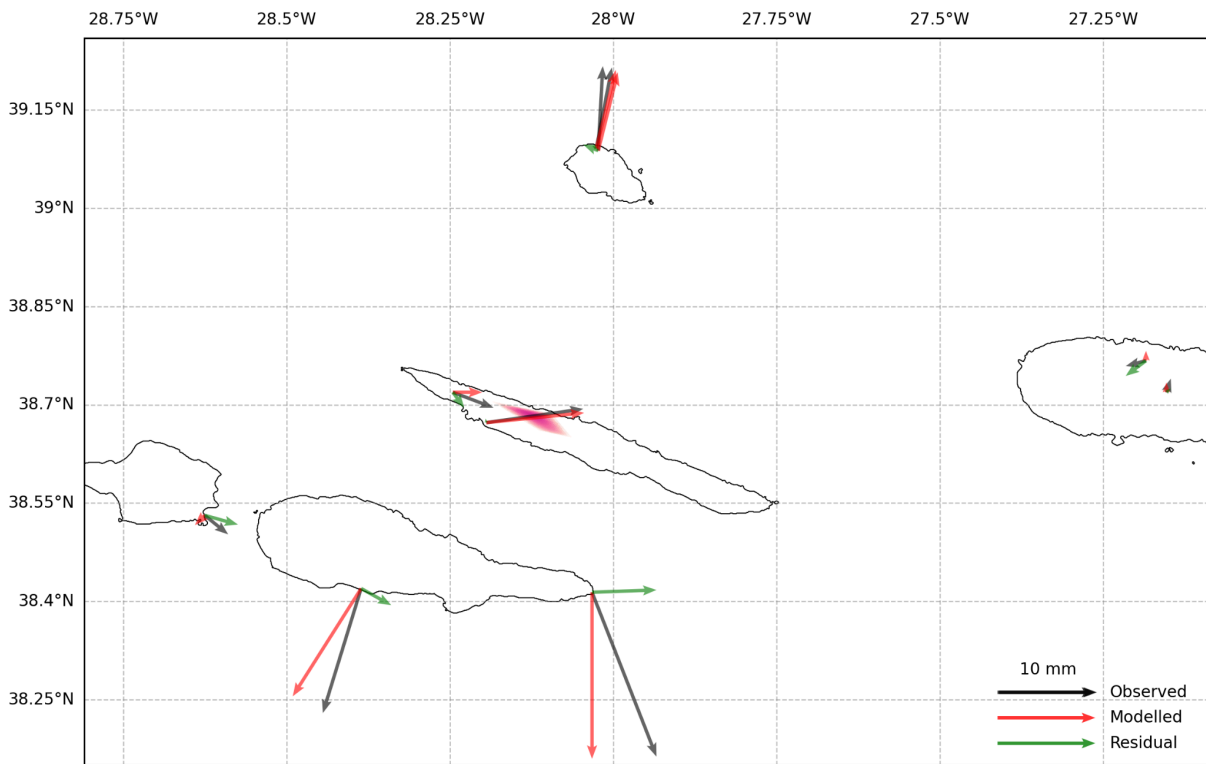
Fig S9: Observed, predicted, and residual GNSS horizontal displacement vectors from our joint BEM dike intrusion model. The dike intrusion is shown in purple.
