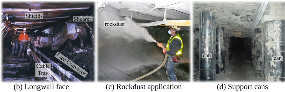
Fig. 1. Longwall mining concept. (a) conceptual diagram of the longwall (modified from [23]), (b) A photograph of a longwall face (modified from [24]), (c) A miner applying rockdust in a gateroad (photo in public domain), and (d) installed secondary support cans (modified from [25]).
