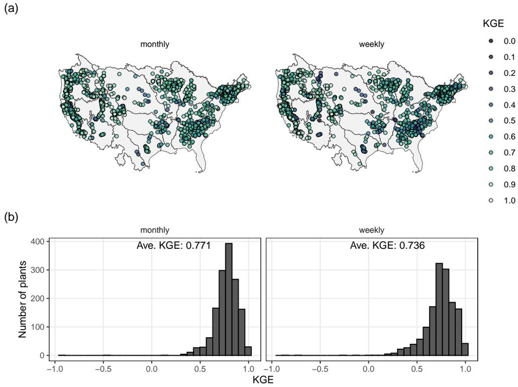
**Figure 3.** KGE values from the B1hydro model for all modeled hydropower plants for both monthly and weekly data.
