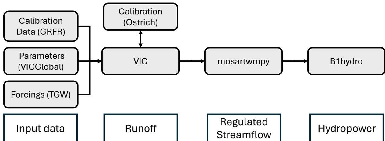
**Figure 1.** Modeling chain used to develop hydropower estimates. The grey boxes indicate models or datasets, and the white boxes indicate the major output from each step of process.
