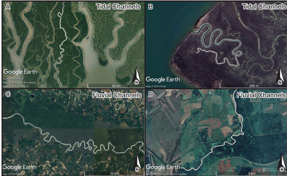
Figure 1: Examples of tidal channels and digitized planforms in: A) Ganges-Brahmaputra, Bangladesh ; B) Brussa, Italy; and fluvial channels and digitized planforms of the C) Congaree River, South Carolina, USA; and D) Latorica River, Slovakia. Note the widening of the tidal channels in the seaward direction in A and B. Digitized banks shown by the white lines. Image Credits – Google Earth V 7.3.6.10201 – A: (1/11/2023) 45Q 783344.84 m E, 2441992.03 m N, Eye altitude: 67.72. Airbus, Maxar Technologies, TerraMetrics 2024, earth.google.com [10/8/2024]; B: (2/20/2024) 33T 342377.00 m E, 5056617.19 m N, Eye Altitude: 736 m. Airbus 2024, earth.google.com [10/8/2024] C: (6/14/2024) 17S 516492.90 m E, 3742013.75 m N, Eye altitude 29.78 km. Airbus 2024, earth.google.com [10/8/2024]; D: (6/12/2020) 34U 565715.29 m E, 5373520.49 m N, Eye altitude: 8.71 km. Eurosense/Geodis Slovakia 2024, earth.google.com [10/8/2024]
