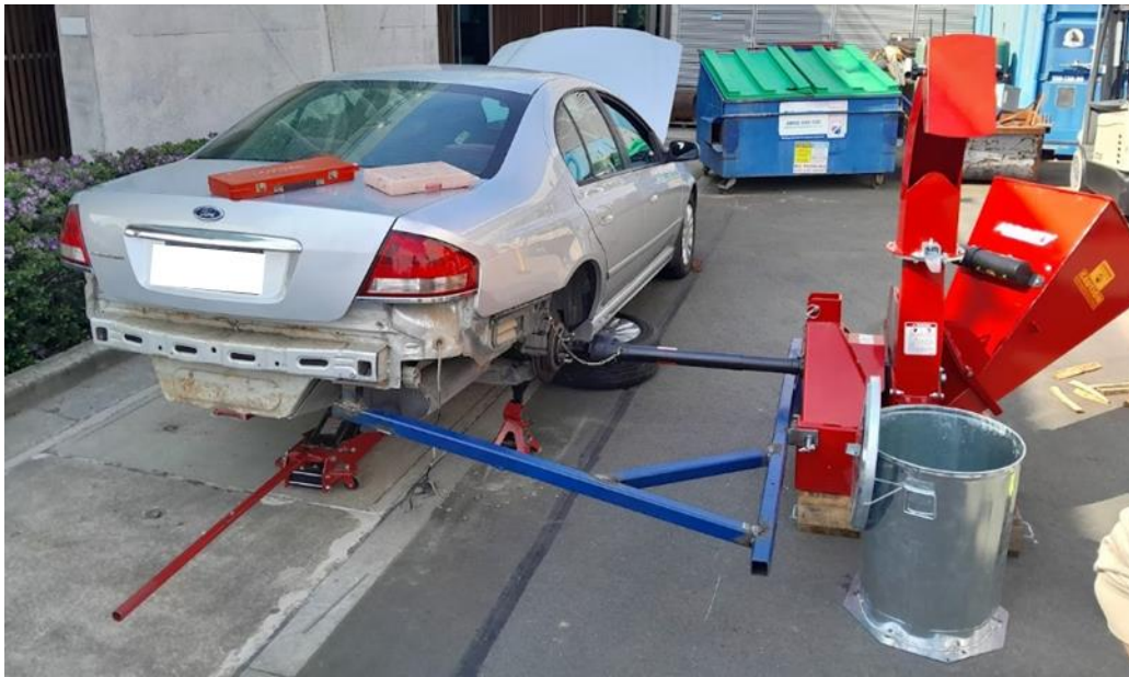
Figure 5: Photograph of the modified vehicle on jackstands and with rear wheels removed, connected to the red woodchipper by the black PTO. The blue steel sections are the moment-restricting frame.
