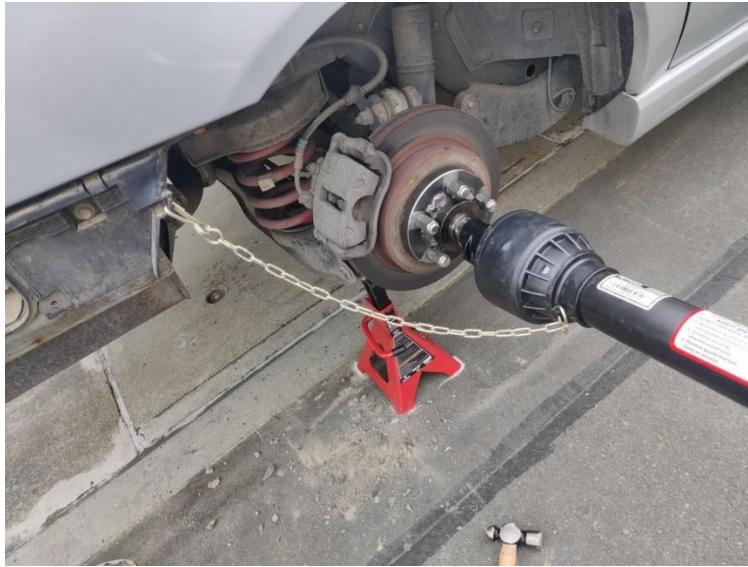
Figure 4: Hub spline adapter mounted to PTO shaft for connecting vehicle's driving wheel to external machinery.
