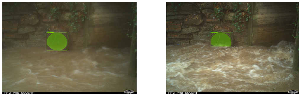
Fig 1. Model capturing an empty outlet (left) and the empty area of the partially filled culvert (right)
