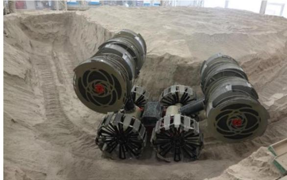
**Figure 3.** RASSOR uses counter-rotating bucket drums to scoop regolith. Reversing the rotation direction on the drums causes regolith to dump out. The relatively narrow openings in the bucket drums prevent large rocks from being collected; thus, beneficiation is inherent to its operation. Credit: NASA/KSC/Mueller et al., 2019.
