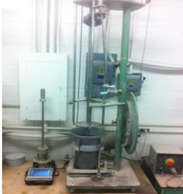
Figure 4. Compaction equipment used for molding a specimen with SCA
