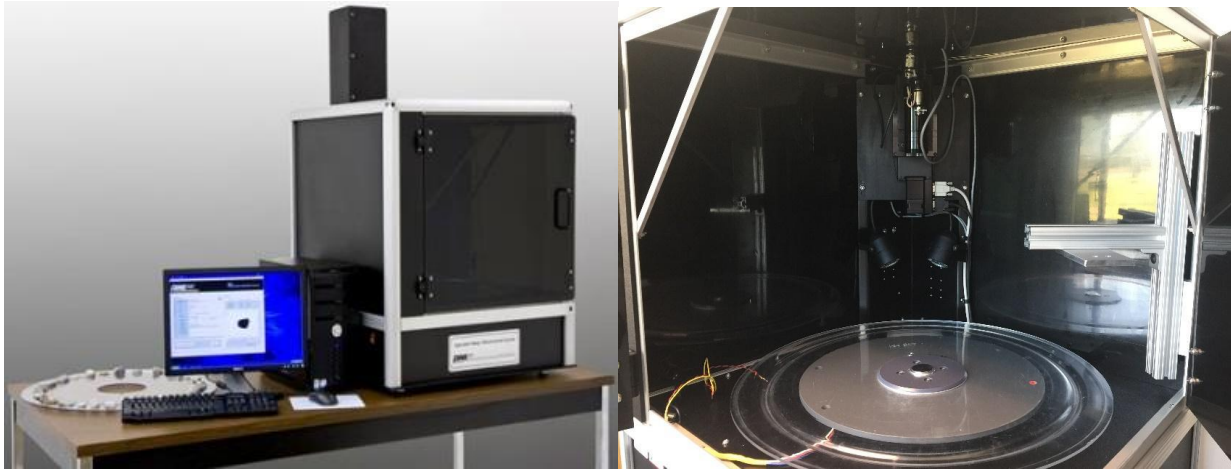
Figure 9. (a) Aggregate Imaging Measurement System (AIMS) Test device; (b) AIMS Camera System
