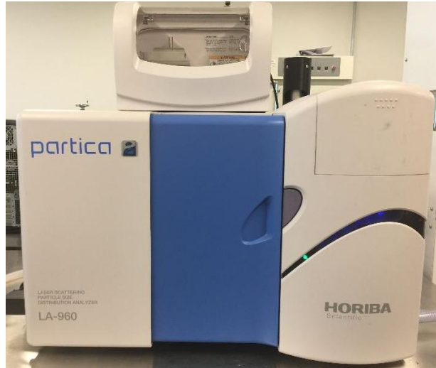
Figure 7. HORIBA LA-960 Laser Particle Size Analyzer
