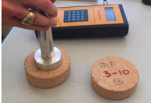
Figure 8. Adek Percometer measuring the dielectric constant of compacted base samples
