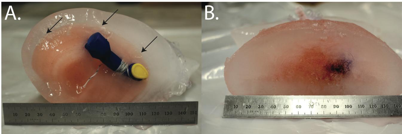
**Fig. 5.** Samples after freezing and saw cut in cross section. A. Set point temperature  $-60\text{ }^{\circ}\text{C}$ , freshwater; B. Set point temperature  $-10\text{ }^{\circ}\text{C}$ ; salinity 5 g/l. The freshwater sample shows a region without dye with a sharp boundary (noted with black arrows). The saltwater sample shows a diffuse gradient between regions with higher and lower dye concentrations.
