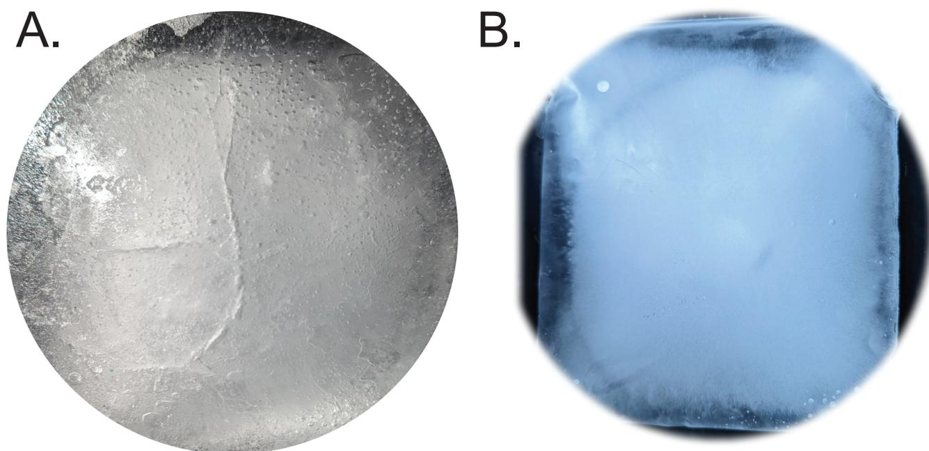
**Fig. 2.** A. Sample with fractures at set point temperature  $-30\text{ }^{\circ}\text{C}$  and salinity  $0.25\text{ g/l}$  (the image spans  $1.7\text{ cm}$ ). B. Sample without fractures at set point temperature  $-30\text{ }^{\circ}\text{C}$  and salinity:  $0.5\text{ g/l}$  (the image spans  $2\text{ cm}$ ). Note that the fracturing present at lower salinity (A) has been suppressed by increasing salinity (B).
