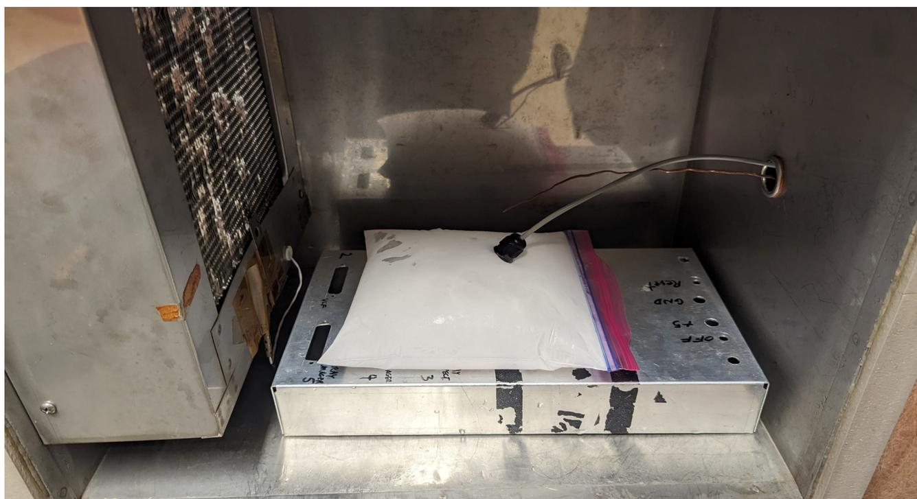
**Fig. 1.** The Associated Environmental Systems Environmental Chamber (Model SK-2101) with frozen ice sample, hollow aluminum stand, thermocouple temperature sensor, and pressure sensor with cable gland.
