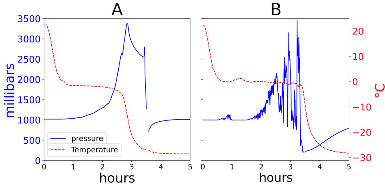
**Fig. 3.** In situ temperature and pressure during freezing, demonstrating difference between saltwater and freshwater experiments. A. Experiment with set point temperature  $-30^{\circ}\text{C}$  and salinity 6 g/L. B. Experiment with set point temperature  $-30^{\circ}\text{C}$  and salinity 0 g/L.
