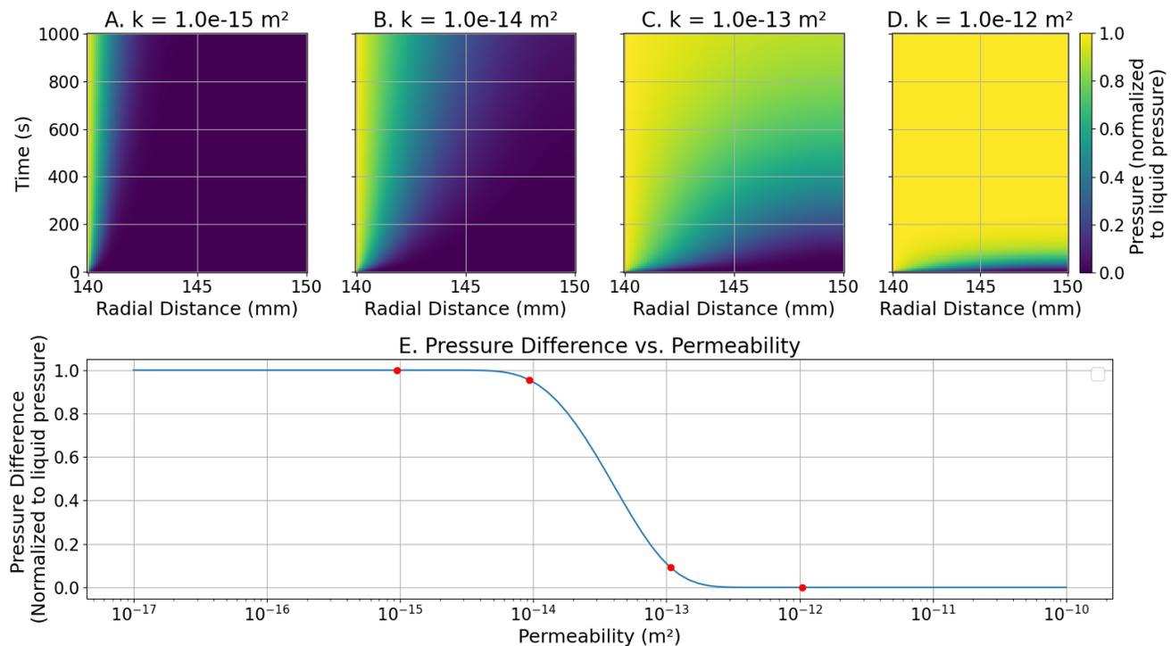
**Fig. 7.** A-D. Numerical calculations of the water pressure in a poroelastic ice shell with different hydraulic permeabilities. The liquid phase region extends from 0 mm to 140 mm and the ice shell comprises 140 mm to 150 mm. E. pressure differences at the last time step between the liquid-ice boundary at 140 mm and the outer shell boundary at 150 mm as a function of permeability. The red dots indicate the four regimes of permeability shown in panels A-D in sequential order.
