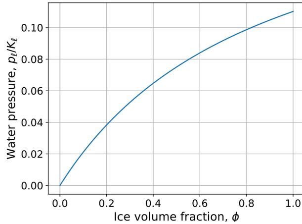
**Fig. 6.** Water pressure within an unfrozen sphere of liquid water surrounded by an expanding icy shell, given as a function of ice volume fraction.
