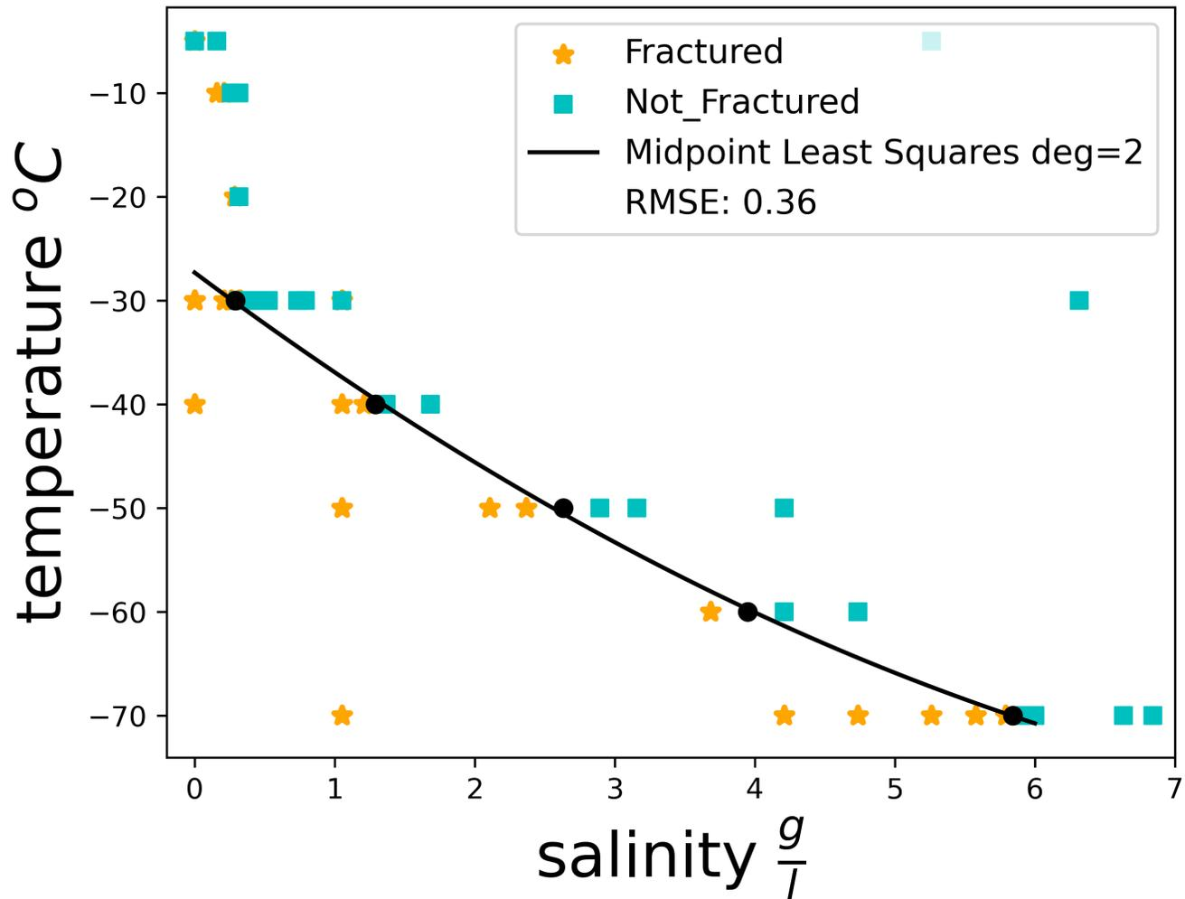
**Fig. 4.** The fracture stability TS curve. Orange stars show experiments where fractures were present and teal squares show experiments where fractures were absent. For each temperature where experiments were conducted, the black circles denote the midpoint between the salinities where fractures were and were not observed; the black curve connects the black dots with a parabolic polynomial.
