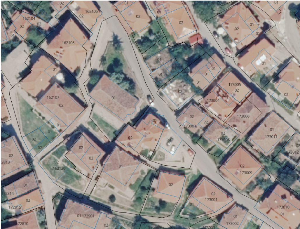
Figure 8. Transformation of the 1925 cadastral map into vector format using the trained GAM. Buildings from the old map are outlined in blue, while land parcels are shown in black. The numbers inside the buildings indicate the number of floors, and the parcel codes correspond to the six-digit numbers (both from the 1925 map). The background is an orthophoto map of the area from the Greek National Cadastre (2015).
