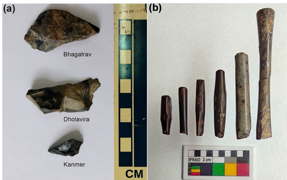
Figure 2. (a) Ernestite stones from Dholavira, Bhagatrav, and Kanmer studied in this work. Note the compositional variations between different samples, as reflected in their colors. (b) Ernestite drill bits from Kanmer. Note the compositional variations. The first and third samples have been used for isotopic analyses.
