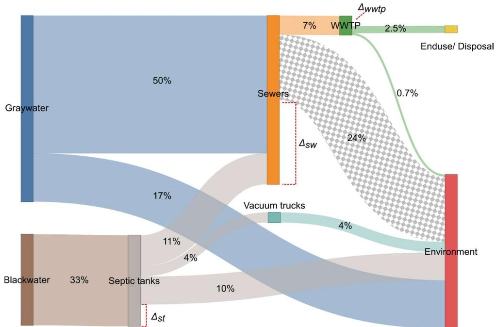
**Fig. 2.** COD mass flow in Hanoi, Vietnam. The percentage flow is expressed in relation to the total COD generated from blackwater and graywater in the SSC.
