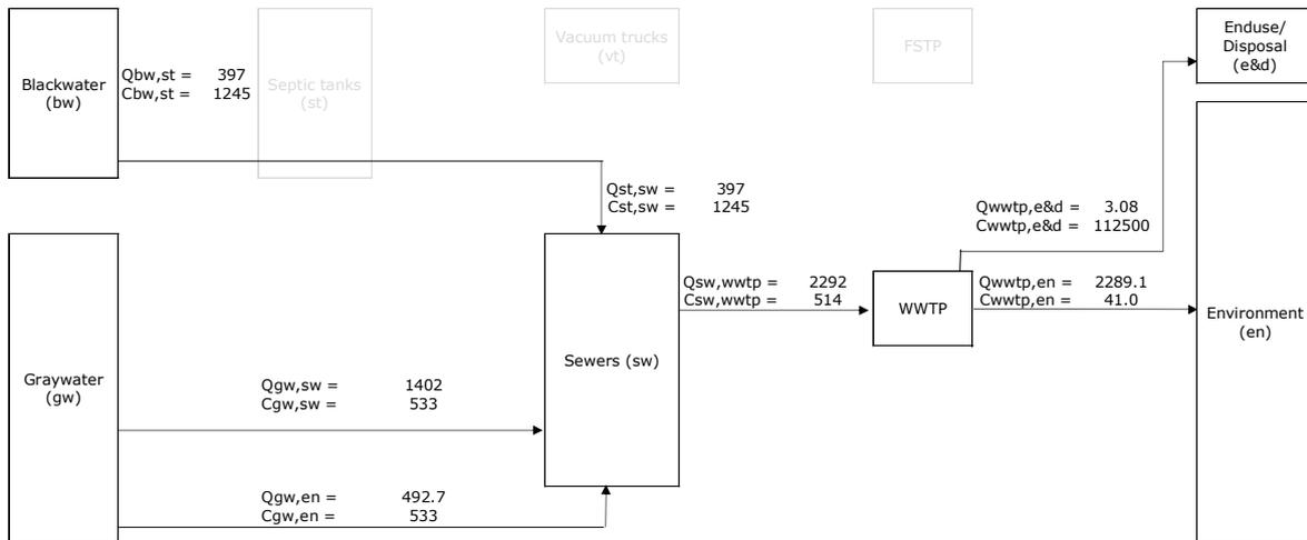
Figure S 1-6 Mass balance diagram for scenario B\*
