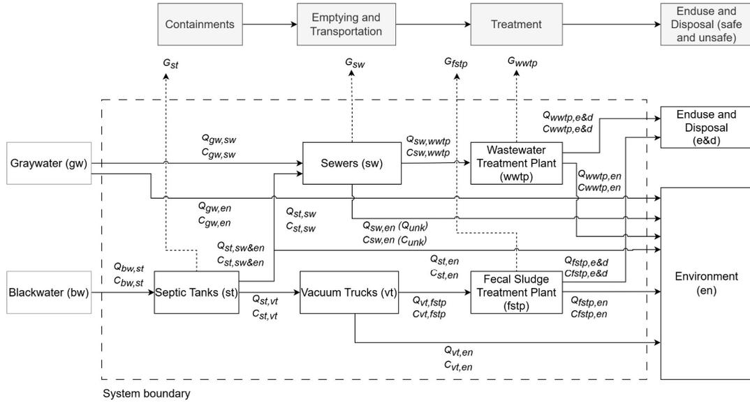
**Fig. 1.** Diagram showing the flow rates ( $Q$ ) and chemical oxygen demand (COD) concentrations ( $C$ ) of the sanitation service chain (SSC), including the system boundary.  $Q_{i,j}$  denotes the flow rate from component  $i$  to  $j$ .  $C_{i,j}$  denotes the change in COD concentration from component  $i$  to  $j$ .  $G_i$  denotes gases emitted from component  $i$ .
