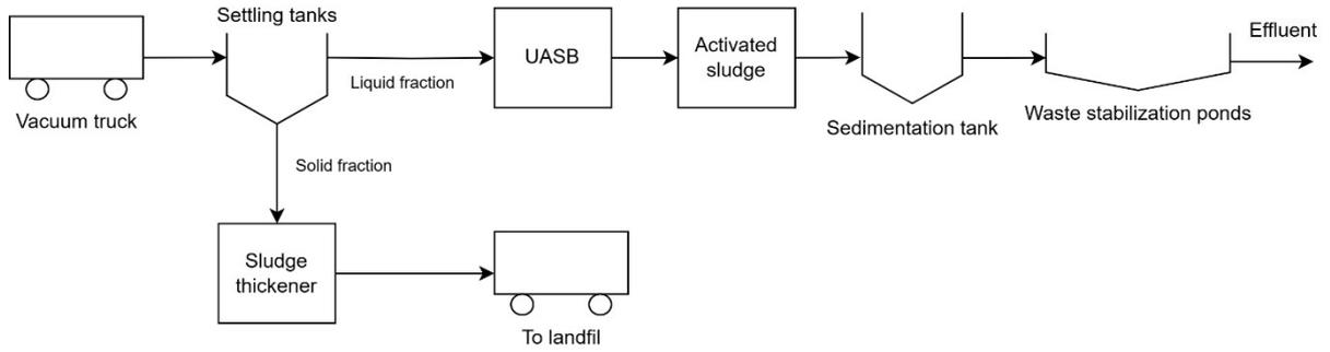
Figure S6–1 Current Cau Dzien FSTP process diagram (Brandes et al., 2016)
