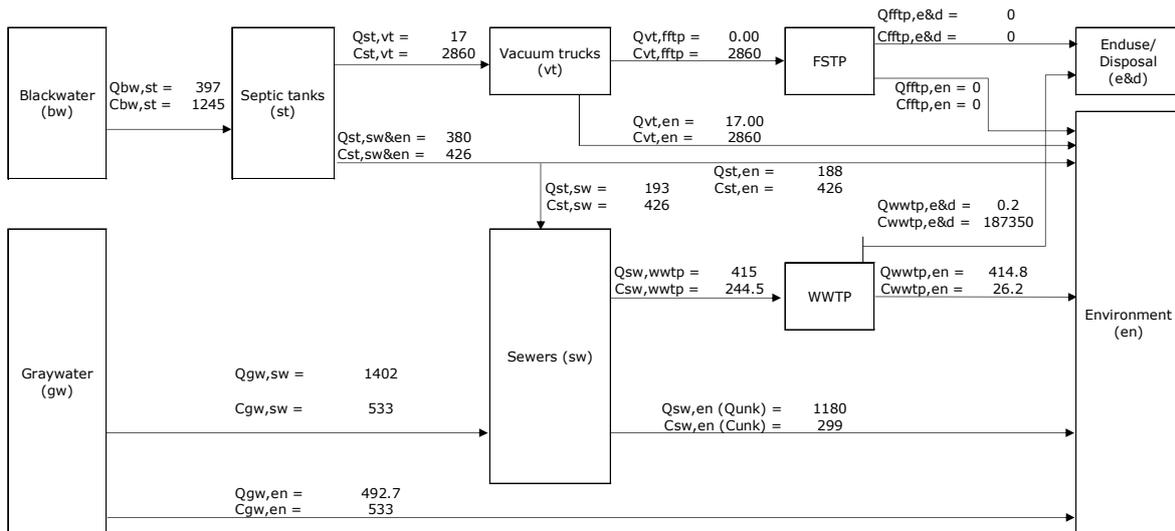
Figure S1-3 Mass balance diagram for scenario A
