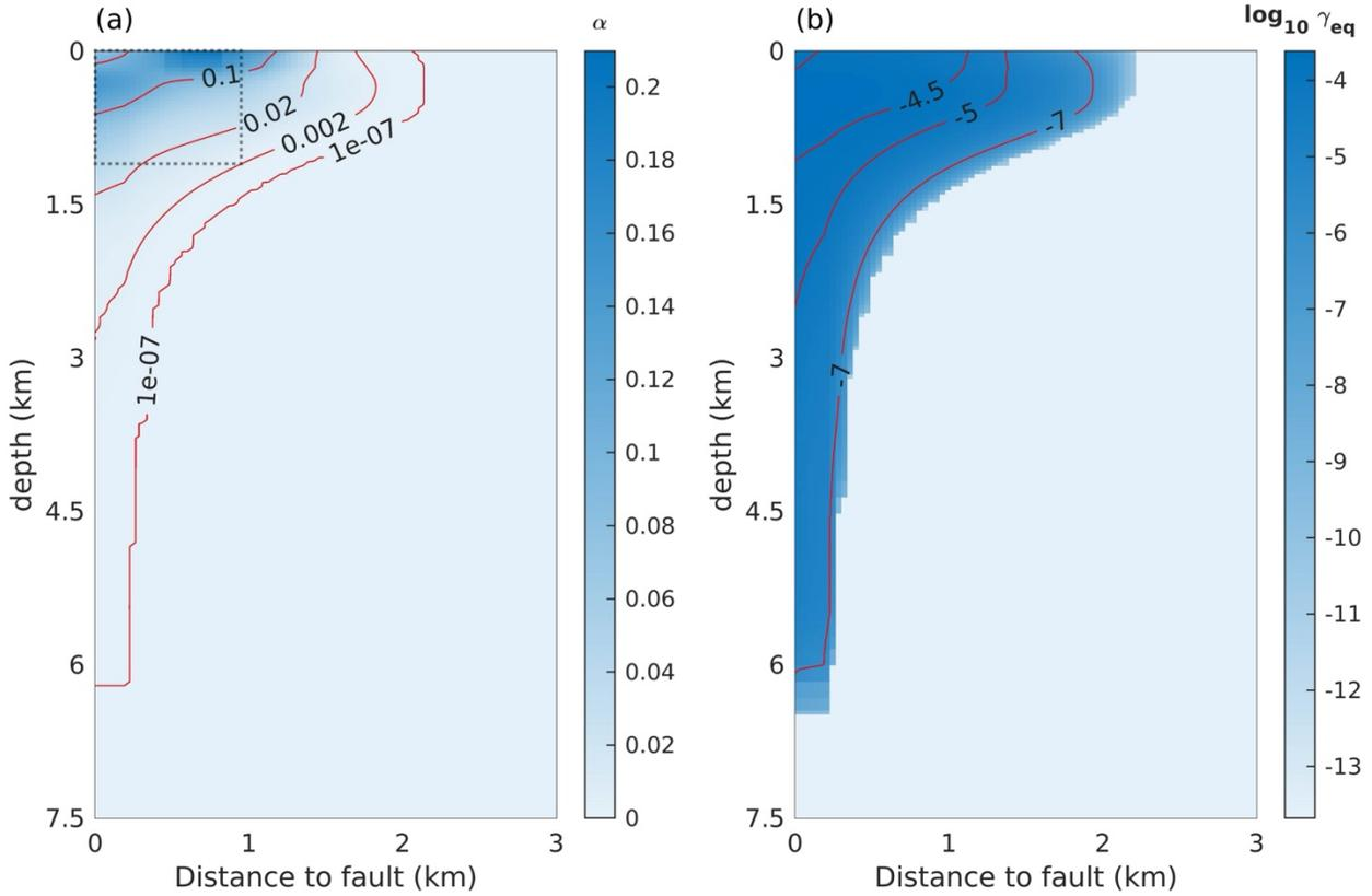
512 **Fig. 8** Spatial distribution of (a) damage variable and (b) equivalent cumulative plastic strain ( $\gamma_{eq} = \sqrt{\epsilon_{ij}^p \epsilon_{ij}^p}$ )
