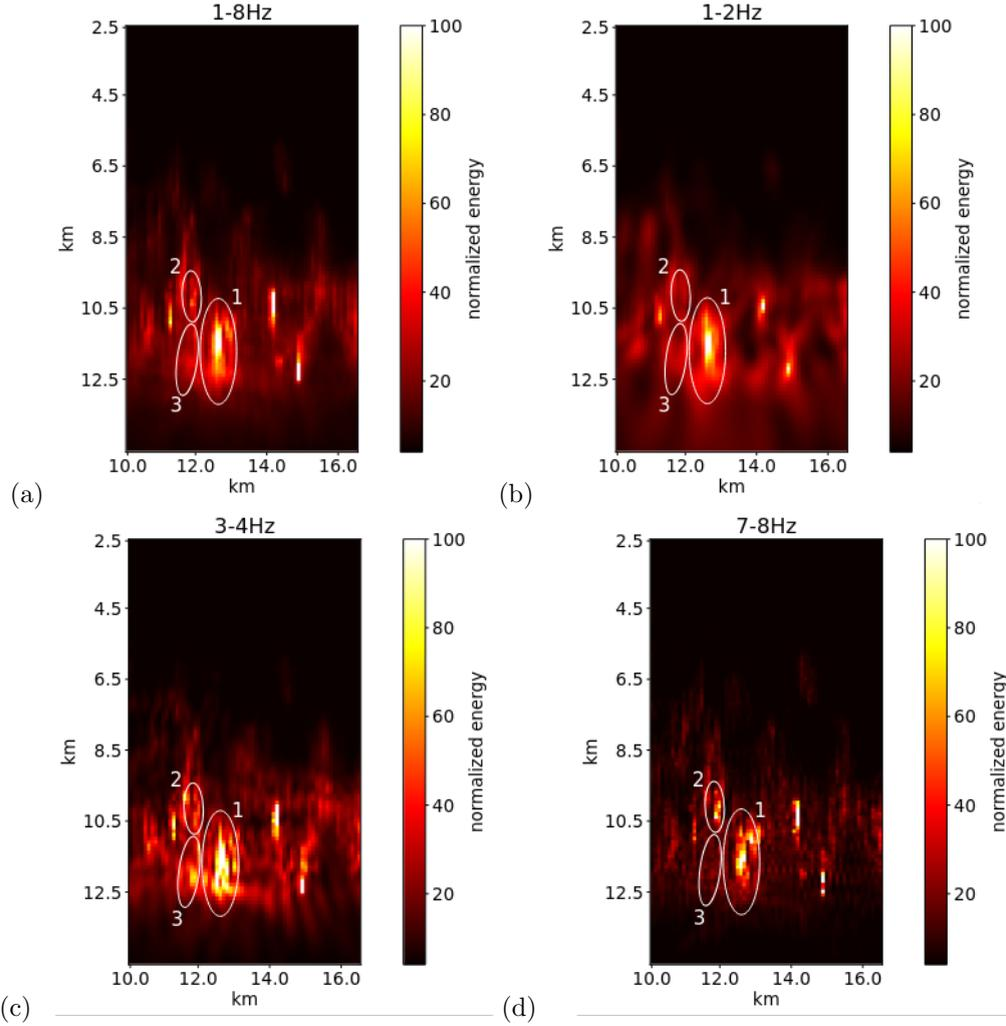
**Figure 6.** Maps of the normalized coda energy generated by vertical component force sources computed after filtering signals in different frequency ranges: (a) All frequencies, (b) 1-2Hz, (c) 3-4Hz, (d) 7-8Hz.
