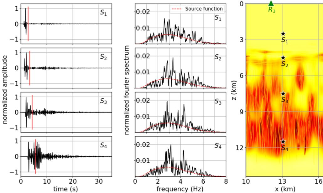
**Figure 3.** Vertical displacement seismograms (left frames) and their Fourier amplitude spectra (right frames) recorded at receiver number 3 ( $x=12.5\text{km}$ ) generated by four vertical force sources located at  $x = 13.0\text{km}$  and different depths:  $z_{S_1} = 2.5\text{ km}$ ,  $z_{S_2} = 4.5\text{ km}$ ,  $z_{S_3} = 7.5\text{ km}$ ,  $z_{S_4} = 11.5\text{ km}$ . Dashed red lines show the spectrum of the source time function.
