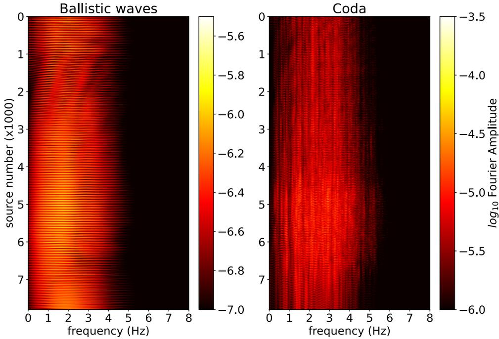
**Figure 4.** Spectra of vertical displacement generated by a vertical force recorded at receiver number 3 for all the sources, sorted by source number. On the left, the spectrum obtained considering only the ballistic arrivals; on the right, considering only the coda. The ballistic part appears much smoother than the coda part, indicating that the peaks in the signals are related to the waves scattered in the structure.
