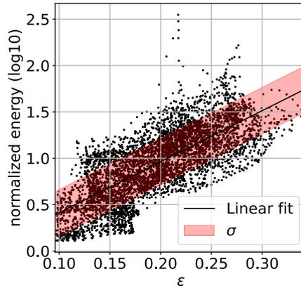
**Figure 5.** Logarithm of the normalized coda energy as a function of  $\epsilon$  in the source region for all source-receiver pairs. Vertical component force sources located in points with  $\epsilon > 0.1$  were considered.
