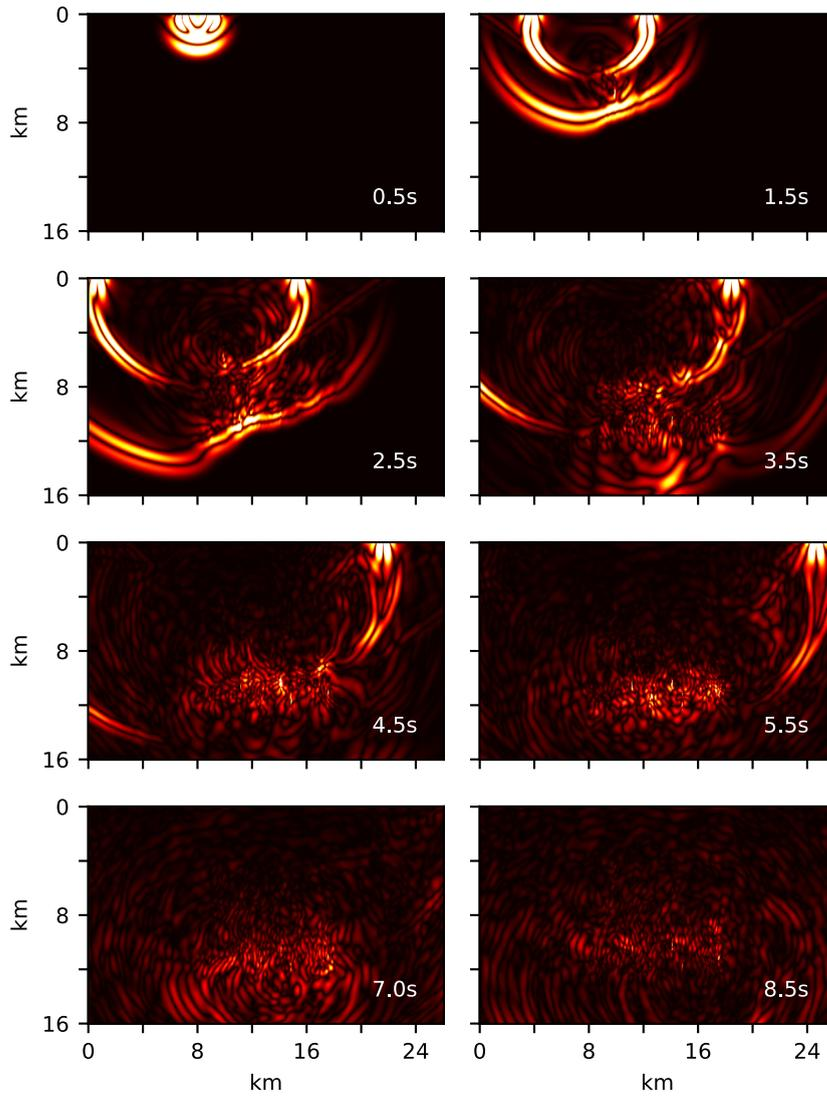
**Figure 2.** Snapshots of the vertical displacement wavefield amplitude generated by a vertical force source located at  $x=8.0\text{km}$ ,  $z = 0\text{km}$ . Times after origin are indicated at bottom-right corners of the snapshots.
