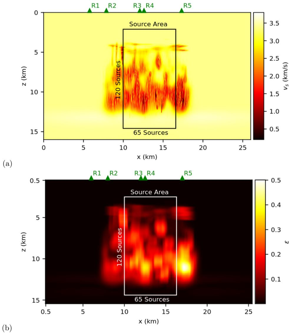
**Figure 1.** Synthetic seismic velocity model. (a) Shear wave velocity. (b) standard deviation of the shear wave velocity fluctuations (equation 1).
