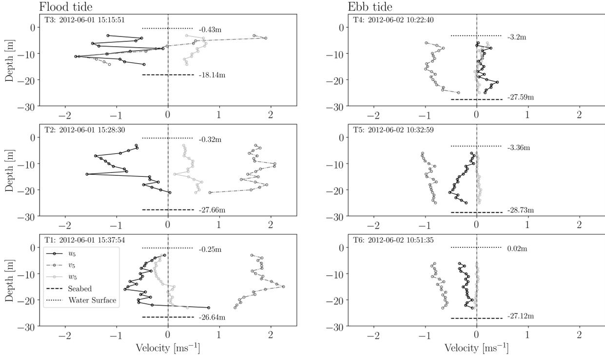
Figure 10: Vertical profiles of time-averaged velocity components ( $u_5$ ,  $v_5$  and  $w_5$ ) from the vessel-mounted ADCP surveys along the stream-wise centre line of Horse Rock during peak flood and ebb tides. Depth is relative to mean water level (MWL).
