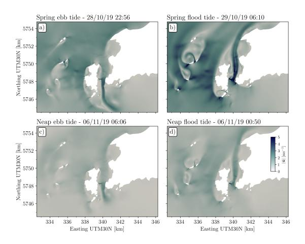
Figure 13: Modelled depth-averaged velocity magnitude  $|\tilde{\mathbf{u}}|$  in the coastal regions surrounding Ramsey Sound during peak ebb and flood tide velocities under spring and neap conditions.
