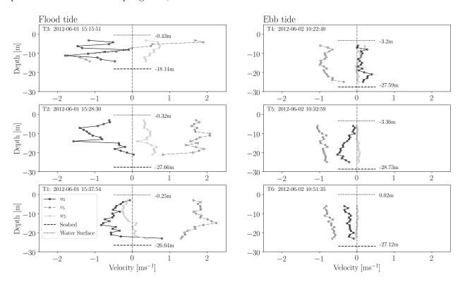
Figure 10: Vertical profiles of time-averaged velocity components  $(u_5, v_5 \text{ and } w_5)$  from the vessel-mounted ADCP surveys along the stream-wise centre line of Horse Rock during peak flood and ebb tides. Depth is relative to mean water level (MWL).
