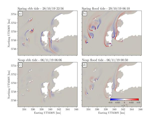
Figure 14: Modelled vorticity around Ramsey Sound and the surrounding waters under different tidal conditions.
