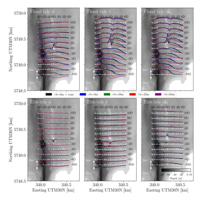
Figure 12: Comparison of spring tide velocity fields in the wake of Horse Rock with 8 (with and without the addition of the cone to the bathymetry), 16, 32 and 64m minimum mesh element sizes  $\wedge h$  around bathymetric features. Grid labelling indicates the distance from the tip of horse rock by the half height diameter of Horse Rock D (m). Internal axes indicates velocity.
