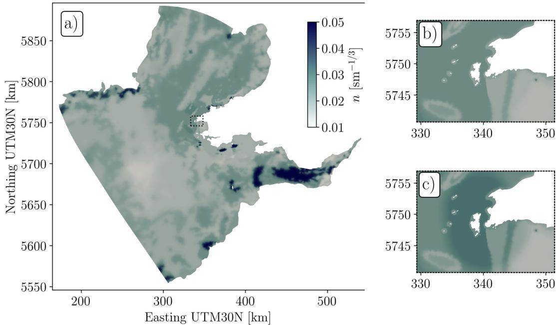
Figure 4: Manning  $n$  coefficient calculated using data from the British Geological Survey interpolated as a variable field denoted by  $N$  onto computational mesh domain. c) indicates variable scaling field  $N^*$ , with Manning coefficient amplified locally to Ramsey Sound at a radius of 10km from Horse Rock, converging towards  $N$  over a further 2km.
