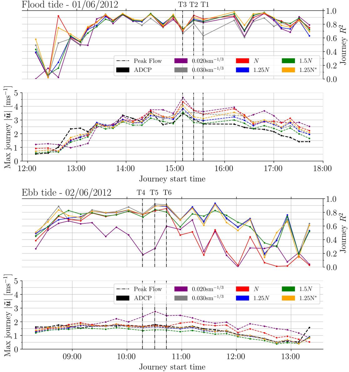
Figure 8: Maximum time- and depth-averaged velocity magnitude  $|\tilde{\mathbf{u}}|_{10}$  from individual boat journeys in vessel-mounted ADCP survey and equivalent  $|\tilde{\mathbf{u}}|$  data sampled from numerical models.  $R^2$  correlation coefficient between ADCP and model data for each journey is also indicated.
