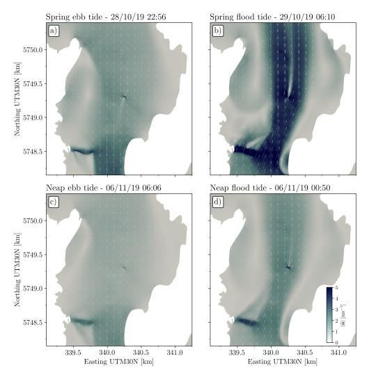
Figure 11: Modelled depth-averaged velocity magnitude  $|\tilde{\mathbf{u}}|$  in Ramsey Sound during peak ebb and flood tide velocities under spring and neap conditions.
