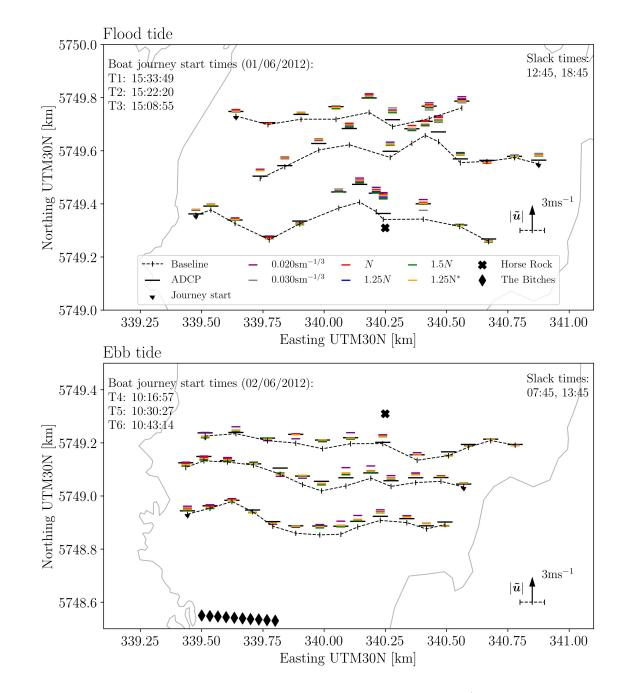
Figure 9: Comparison of depth-averaged velocity magnitude between the numerical model  $\tilde{\mathbf{u}}$  (implementing different Manning coefficient fields) against equivalent 10s time-averaged vessel-mounted ADCP survey data  $|\tilde{\mathbf{u}}_{10}|$  during peak ebb and flood flows (as indicated on Fig. 8). Vertical distance of ADCP and model data from the baseline (also sample location) indicates velocity magnitude.
