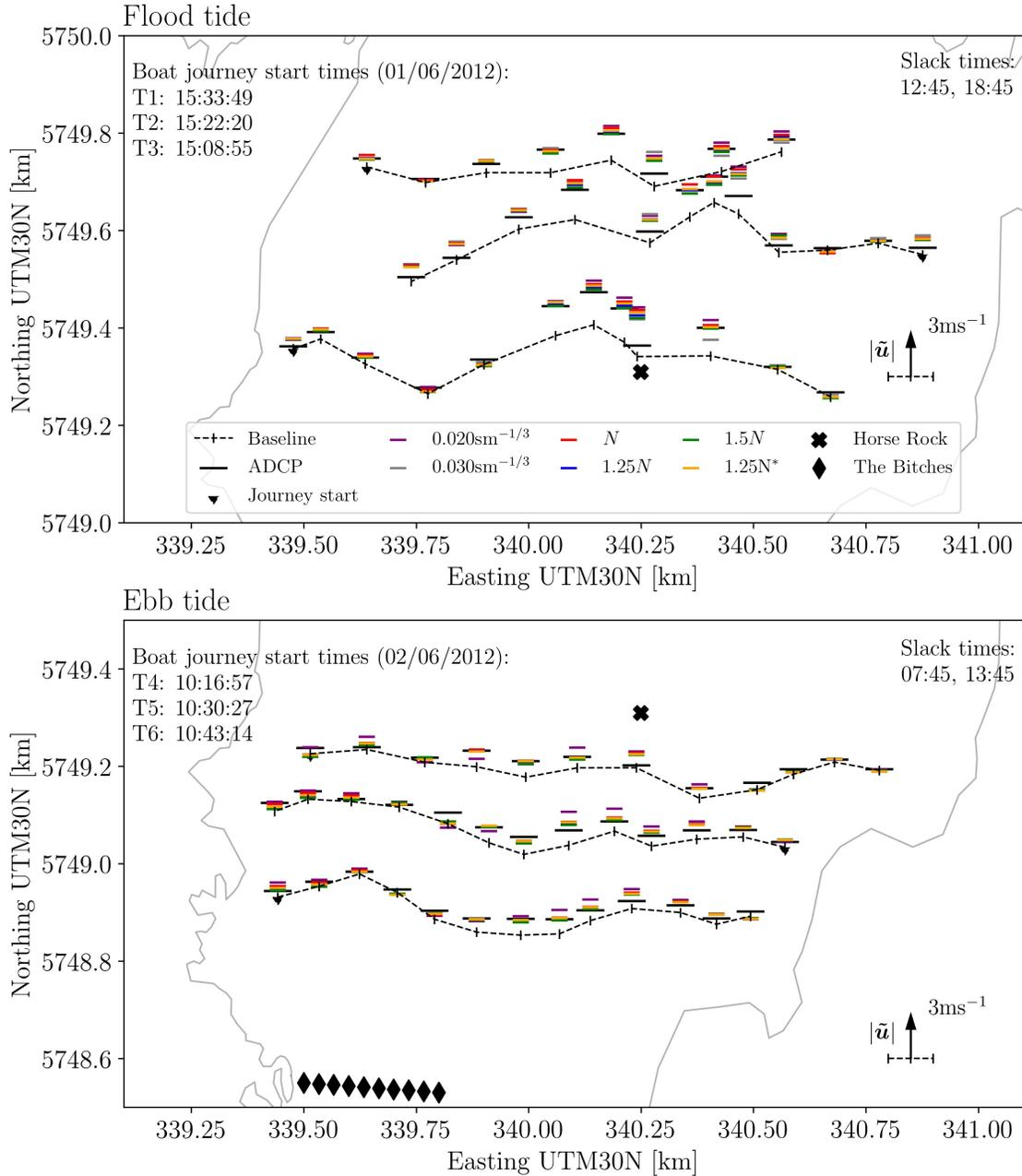
Figure 9: Comparison of depth-averaged velocity magnitude between the numerical model  $\bar{\mathbf{u}}$  (implementing different Manning coefficient fields) against equivalent 10s time-averaged vessel-mounted ADCP survey data  $|\bar{\mathbf{u}}_{10}|$  during peak ebb and flood flows (as indicated on Fig. 8). Vertical distance of ADCP and model data from the baseline (also sample location) indicates velocity magnitude.
