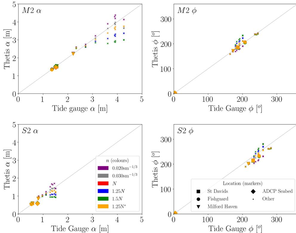
Figure 6: Comparing modelled and measured  $M_2$  and  $S_2$  tidal constituent amplitude  $\alpha$  and phase  $\phi$  at tide gauge locations for different Manning coefficient fields. The near identical values between  $N$  and  $1.25N^*$  obscure results for  $N$ . Tide gauge locations are indicated in Fig. 1a.
