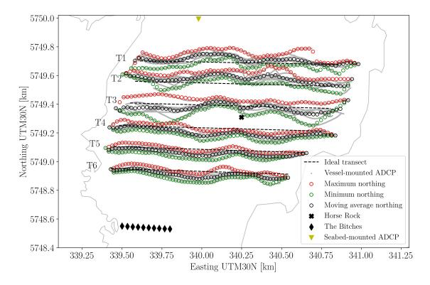
Figure 5: Model data sampling locations are established upon navigation of the ADCP vessel. Along each idealised transect, maximum, minimum and average northing values are determined based on evenly spaced easting bins. Easting coordiantes indicate the centre-point of these bins. ADCP data at transects T1 to T3 was collected as the tide ebbed, and transects T4 to T6 as the tide flooded.
