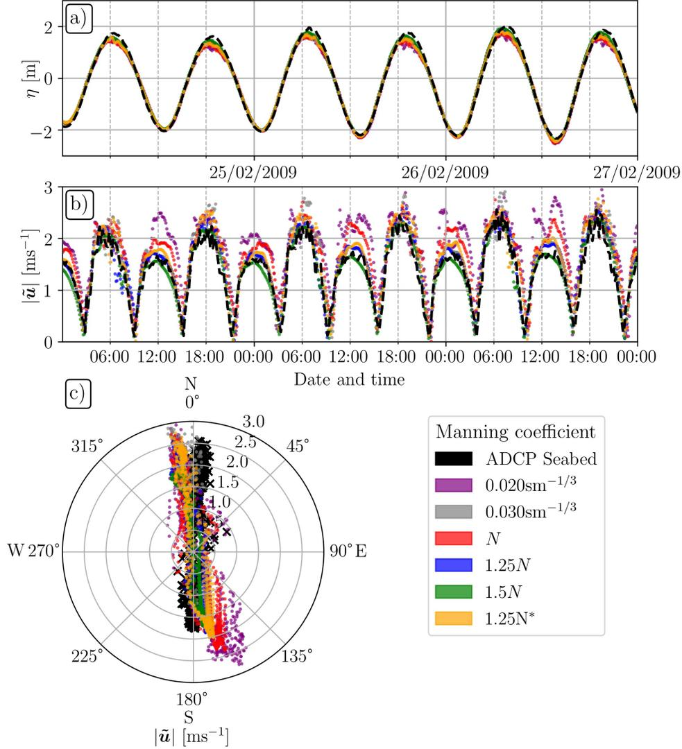
Figure 7: Seabed-mounted ADCP elevation a)  $\eta$  and b, c) depth-averaged velocity  $\tilde{\mathbf{u}}$  measurements (see Fig. 5 for sample location) and *Thetis* model. Data collected during a spring tide over four tidal cycles and displayed as a, b) time-series and c) a polar plot.
