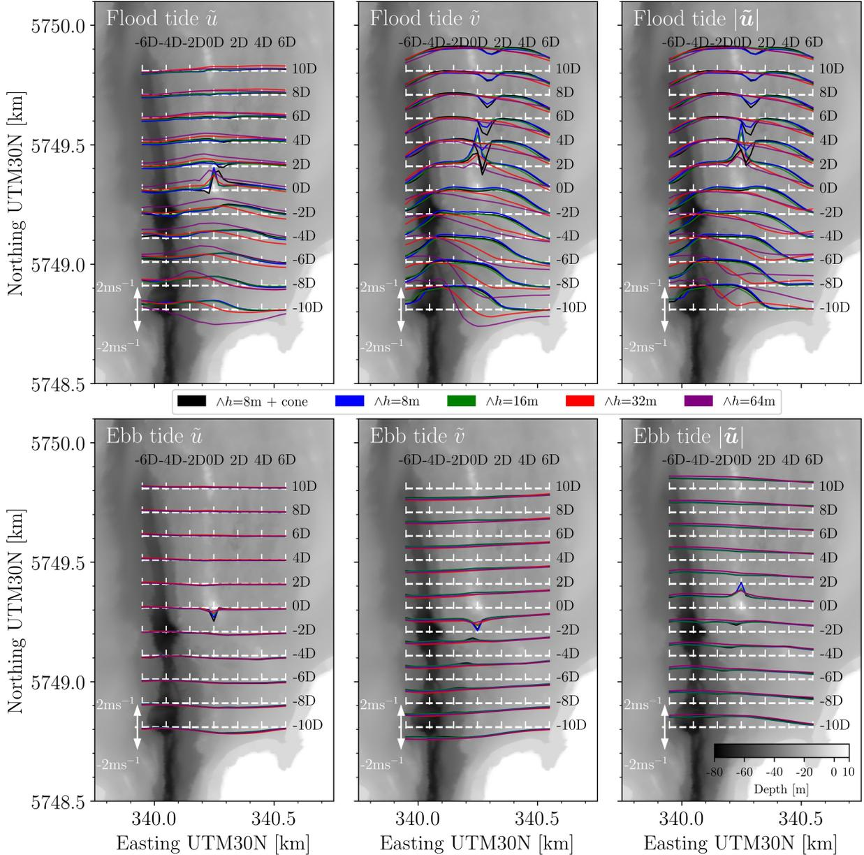
Figure 12: Comparison of spring tide velocity fields in the wake of Horse Rock with 8 (with and without the addition of the cone to the bathymetry), 16, 32 and 64m minimum mesh element sizes  $\Delta h$  around bathymetric features. Grid labelling indicates the distance from the tip of horse rock by the half height diameter of Horse Rock  $D$  (m). Internal axes indicates velocity.
