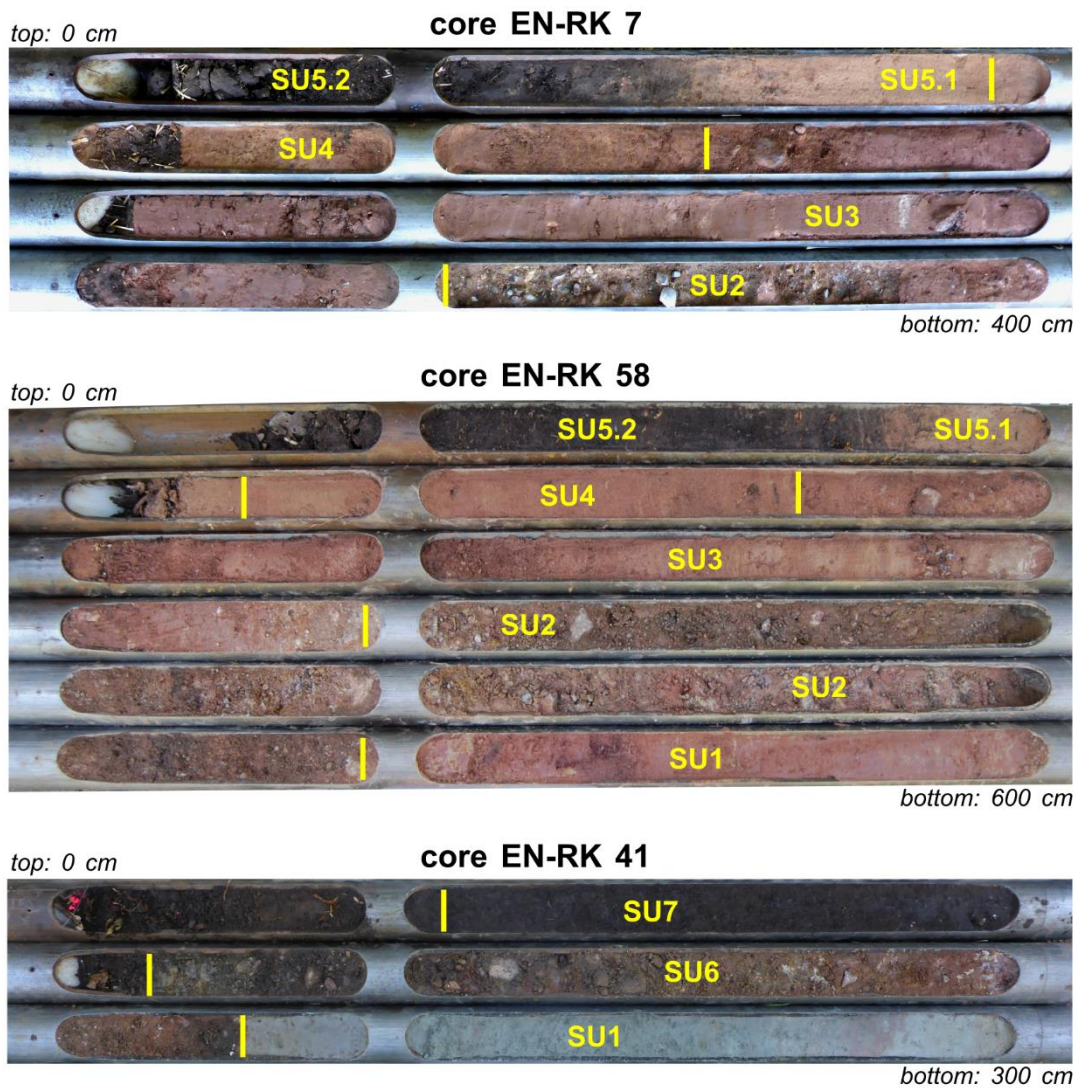
Fig. 4: Photographs of cores representing the Chernozem standard sequences-(EN-RK 7 & 58) and the Black Flood-plain Soil standard sequence (EN-RK 41). The attribution of the different deposits to stratigraphic units (SU) is indicated. Descriptions of SU1 to SU7 can be found in Table 1 and Supplementary Section 3.
