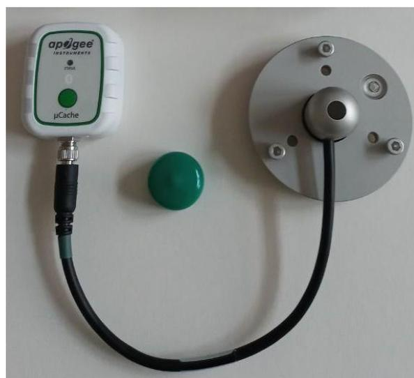
Figure 9: apogee SL-510 upward-looking pyrometer with Bluetooth microcache datalogger
