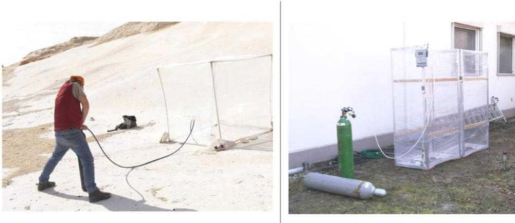
Figure 12: Illustrations of figure 8 were applied in the White Desert location in Egypt and at the Vienna area location. To prevent too strong deteriorations of our measurements it was necessary in both cases to use positions at relatively low wind conditions, which is difficult to have in wintertime
