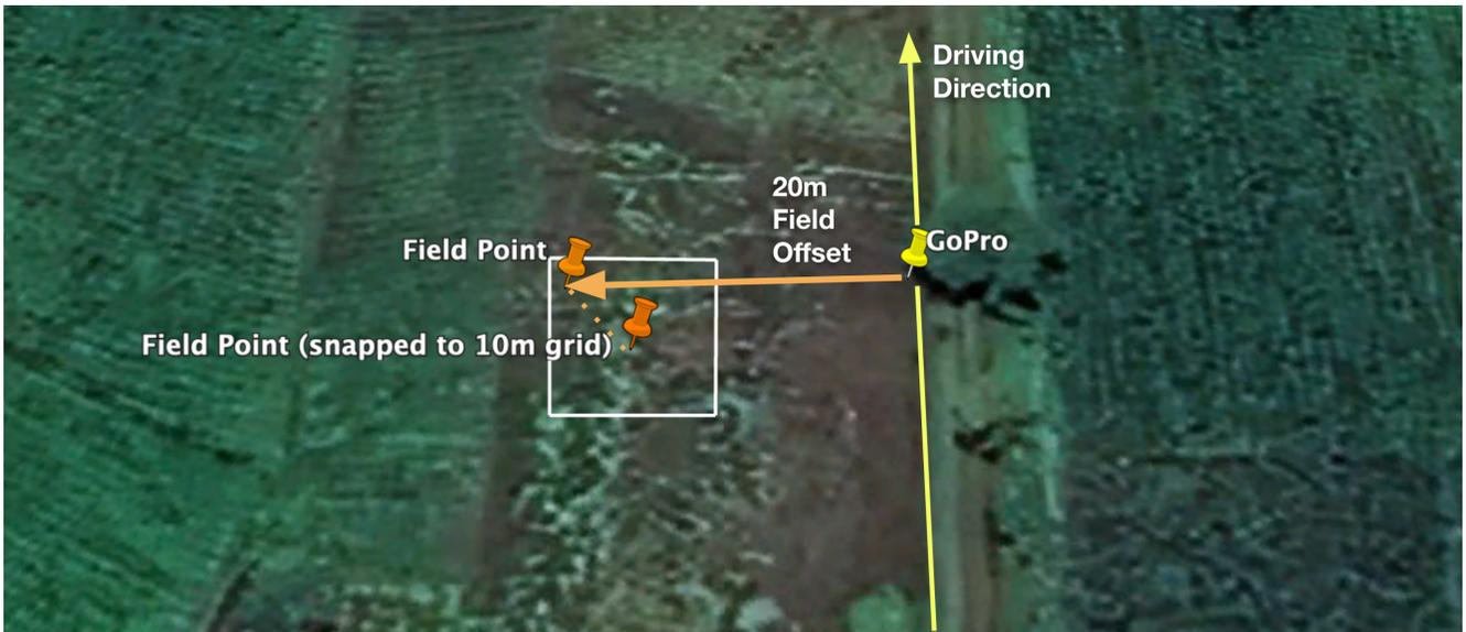
**Figure 4.** Field Offset Algorithm Example.
