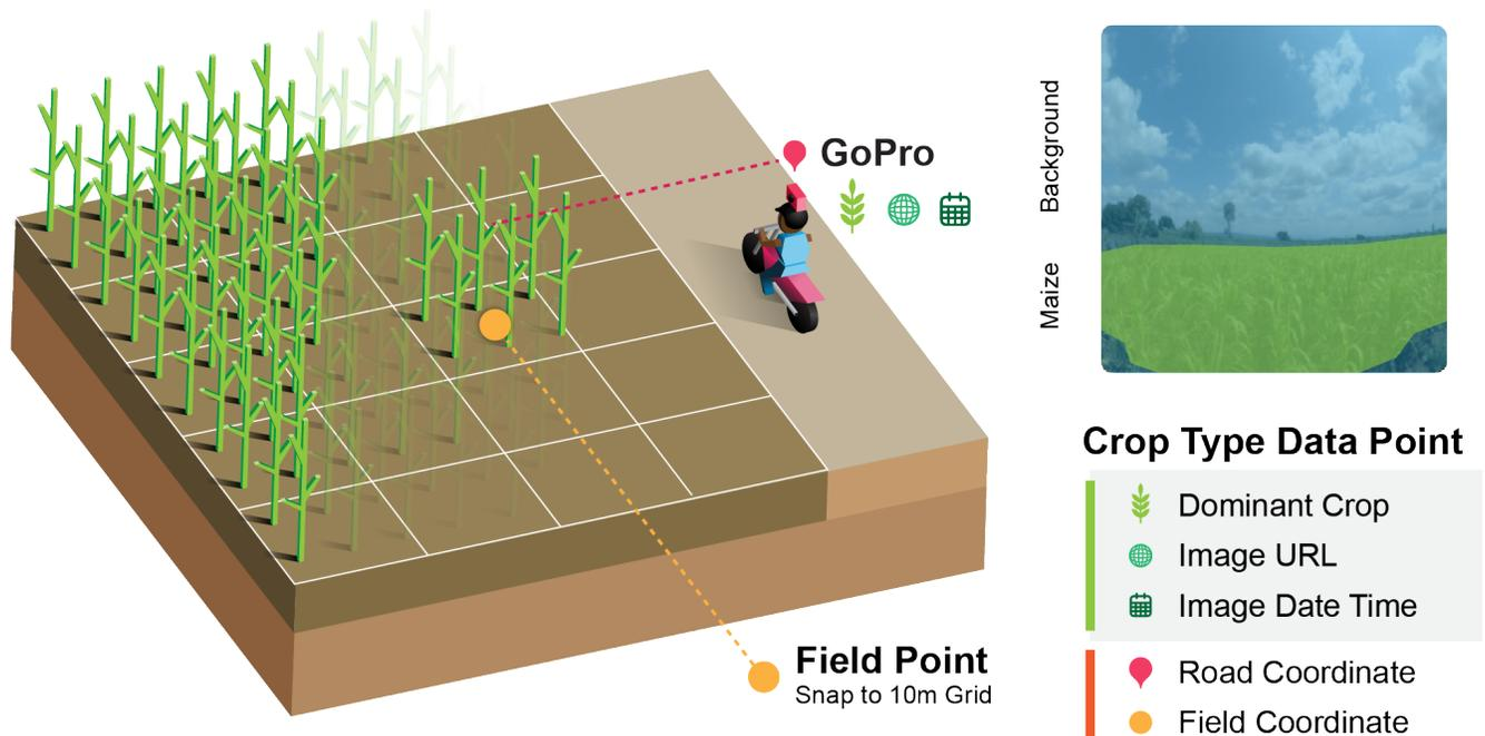
**Figure 1.** Illustration of crop type data generation pipeline. Steps: 1) Field agent with helmet-mounted GoPro drives along agricultural fields, 2) GoPro captures photo of adjacent field (red dotted line) and road coordinate (red point), 3) field coordinate (orange point) is calculated by moving road coordinate 20 meters into field and snapping to 10 meter grid, 4) GoPro photo is used to predict dominant crop.
