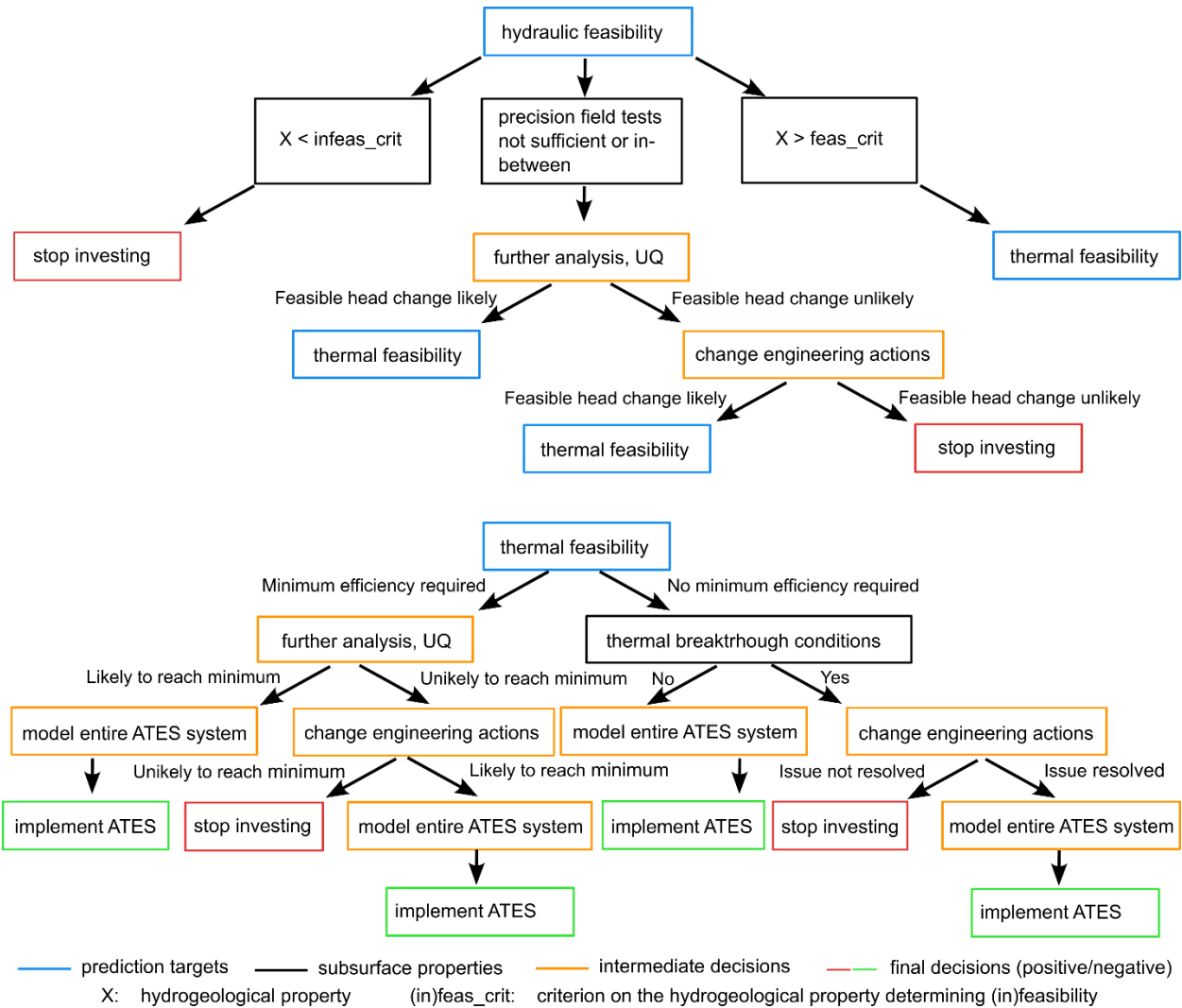
Fig. 15 Decision tree for ATEs in hydrogeological settings where hydraulic feasibility is crucial (primary root node) and thermal feasibility desirable (secondary root node)
