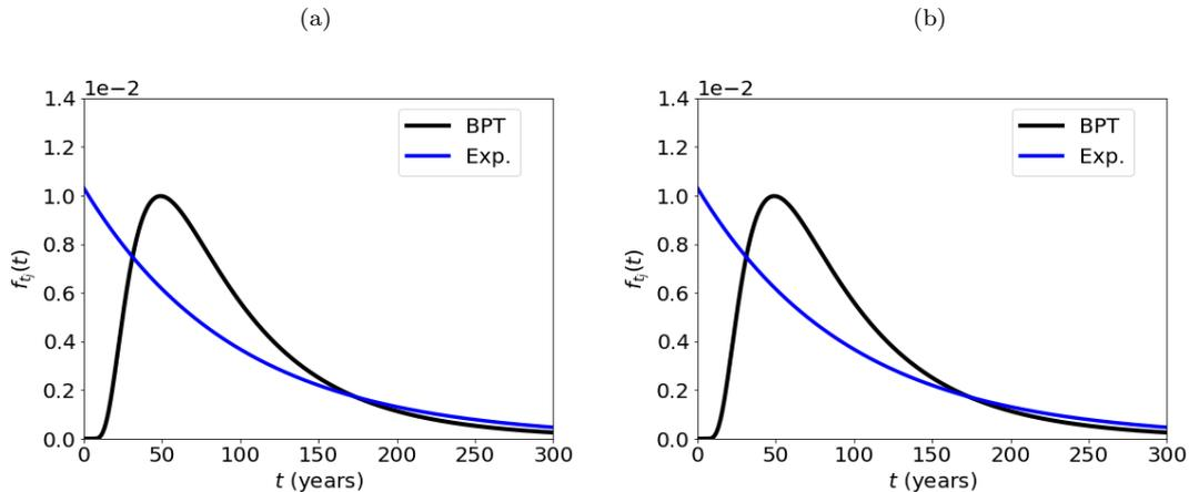
Figure 6: BPT in sections 4 and 5 in black and exponential with equivalent mean in lighter color: (a) probability density function, (b) hazard rate.
