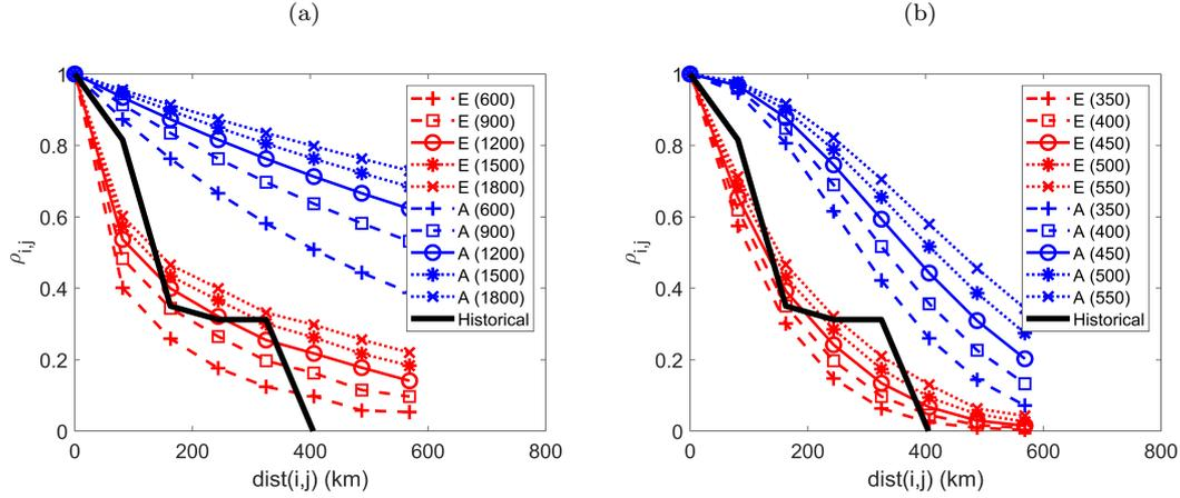
Figure 8: Apparent (A), effective (E), and data-driven (Historical) correlations using different  $\gamma$  values (in parenthesis in km): (a) exponential correlogram, (b) spherical correlogram.
