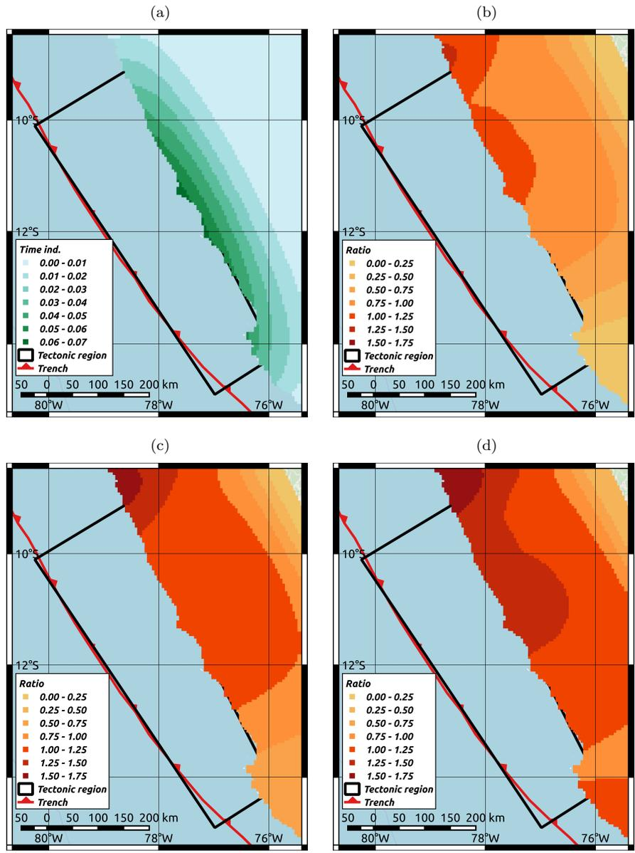
Figure 12: Comparison of  $P[\text{PGA} > 0.4g]$  during 30 years: (a) time independent, (b), time dependent from 2018 to 2047 (c) time dependent with 30 extra years of seismic gap, (d) time dependent with 60 extra years of seismic gap.
