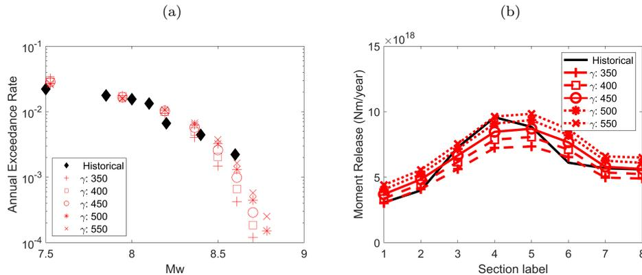
Figure 10: Model benchmark for different spherical correlograms: (a) Magnitude exceedance rates, (b) Average seismic moment (Nm/year)
