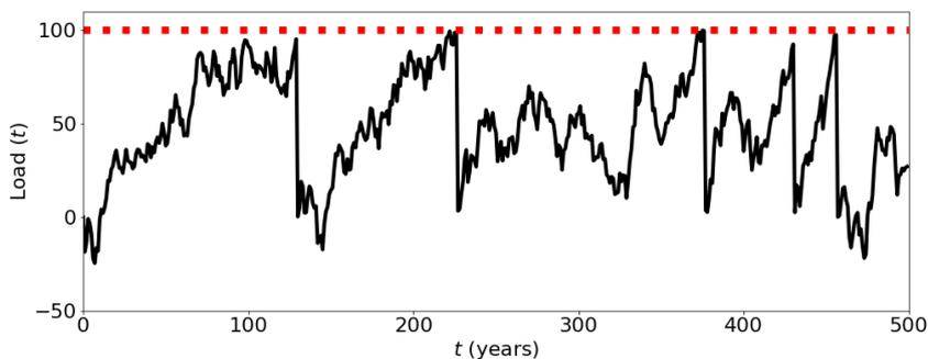
Figure 2: Realization of a load path in Brownian motion for  $\mu = 100$  years and  $\alpha = 0.7$  (aperiodicity). The load resets to zero each time it reaches the threshold shown in the dashed line. The load could have units of tectonic stress or shear stress according to the BRO interpretations in Matthews et al. (2002).
