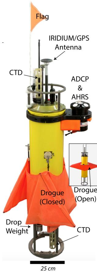
215 FIG. 3. Lagrangian float with a Nortek Signature ADCP and two CTDs. Inset shows a slightly different model
