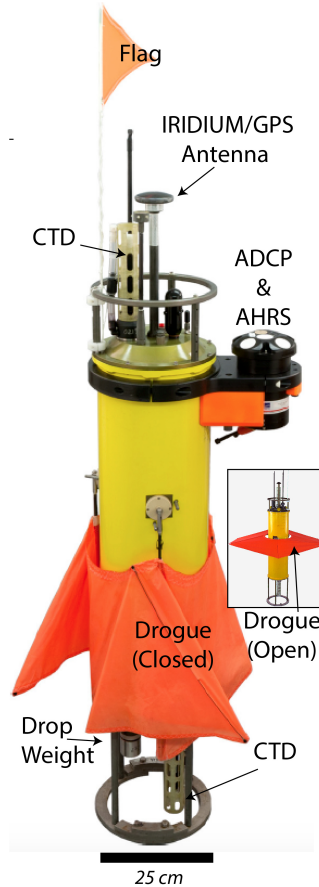
139 FIG. 2. Lagrangian float with a Nortek Signature ADCP and two CTDs. Inset shows a slightly different model 140 of the float with the drogue open. The float displaces about 53 L and is 1.4 m long between the two CTDs; the 141 main tube is 254 mm in diameter.
