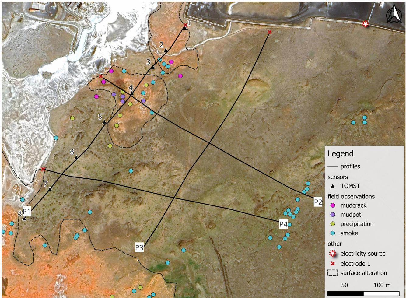
Figure 2: Localization of the ERT profiles (P1-4) and surface observations in the Reykjanes Geothermal Field. The profiles are measured from North to South and West to East, the first electrode is indicated for each profile. The surface alteration is delineated using Google imagery combined with field observations.
