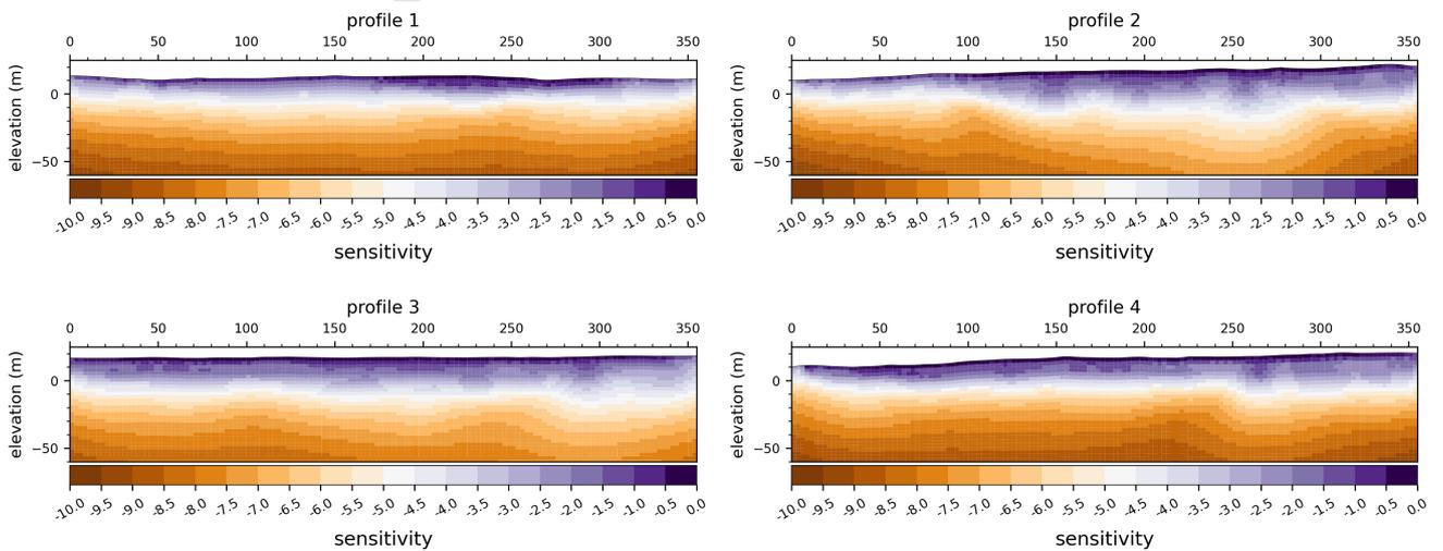
Figure 7: The sensitivity of the four profiles based on the resistivity inversion, a high value reflects that the data is well resolved in the inversion model.
