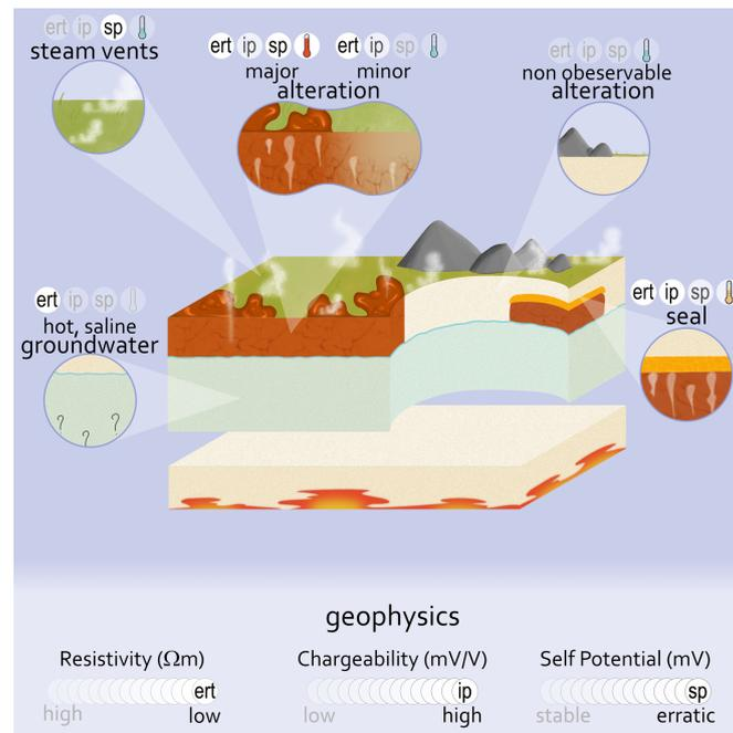
Figure 10: Conceptual model showing the main findings of this research, the different features are indicated alongside the geophysical methods used to identify said features. The brightness of the icons represents the strength of the signal of the parameter. Note that there was no temperature data available in the 'hot saline groundwater' area since our sensors are mounted in the shallow soil.
