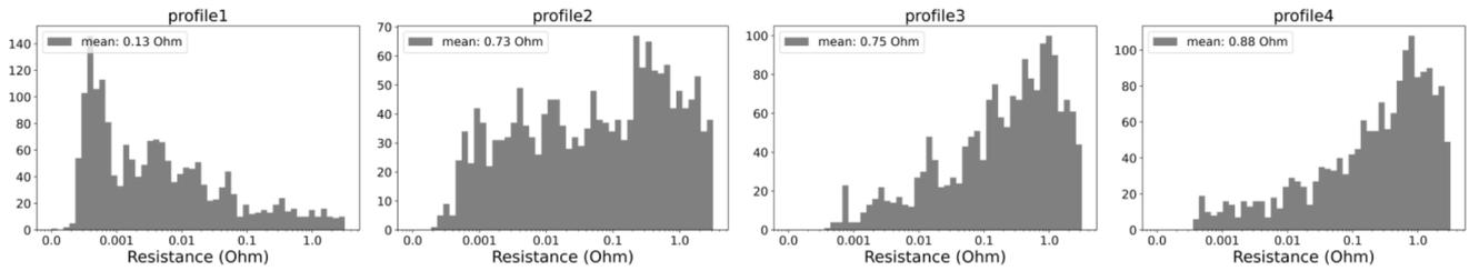
Figure 3: Resistance distribution in the four profiles, the resistance is plotted logarithmically.
