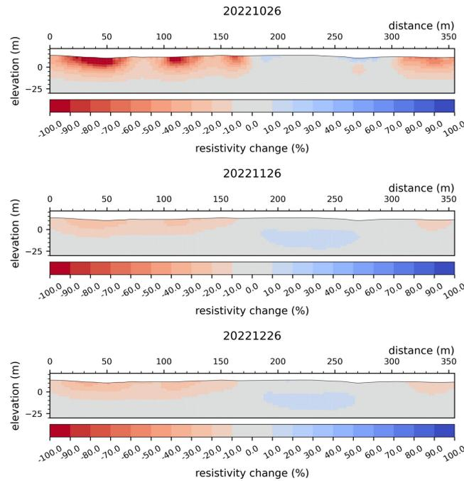
Figure 9: The resistivity change of profile 1 between the measurement shown in Figure 8 and the same profile measured again on 26/10/2022, 26/11/2022 and 26/12/2022. The changes are given in a relative change of resistivity, a positive number reflects an increase and vice versa.
