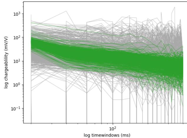
Figure 5: Example of the decay curve analysis for profile 1, a curve is accepted (green lines) when it deviates no more than 60% from a fitted exponential function. Note that the vertical lines represent negative values as they cannot be shown logarithmically.
