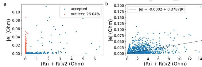
Figure 4: a: example of the data filtering for profile 1, outliers are determined based on the normal/reciprocal discrepancy, with the average resistance plotted against the residual error  $|e|$ . The orange dots represent the points filtered out using the method described by Slater et al. [2000]. b: global error model reconstruction (black line) fitted on the accepted points of the four profiles combined.
