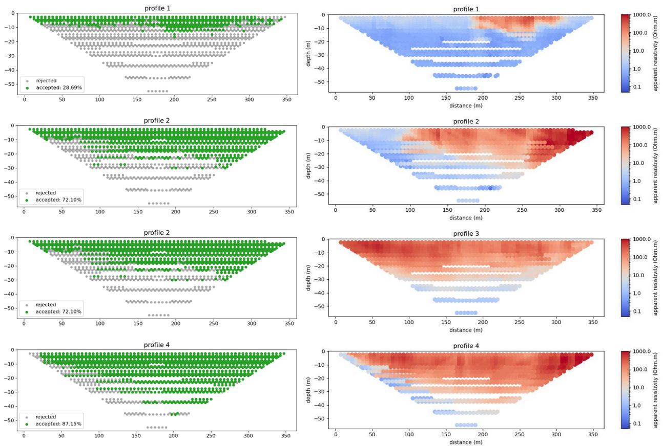
Figure 6: Acceptance rate of the decay curve analysis plotted as a pseudosection, plotted alongside the apparent resistivity, areas where points are rejected coincide with low Resistance.
