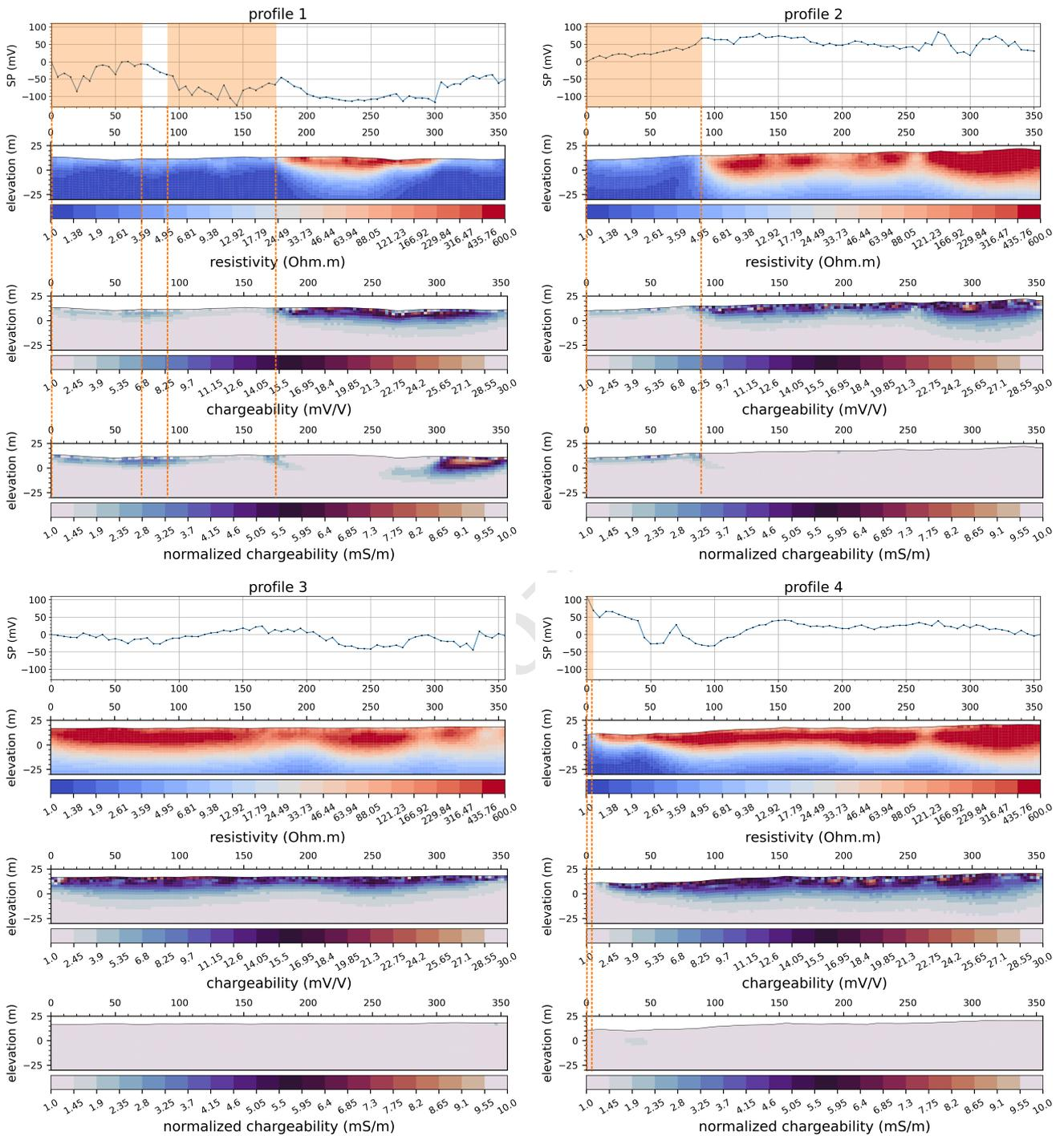
Figure 8: The results from the field campaign, for each profile, there is the corrected SP signal in *mV*, the resistivity in  $\Omega m$ , the chargeability in *mV/V* and the normalized chargeability in *mS/S*. The orange-shaded areas and extended dashed red lines indicate where surface alteration was observed. Profiles 1 and 3 are measured north to south, and profiles 2 and 4 east to west.
