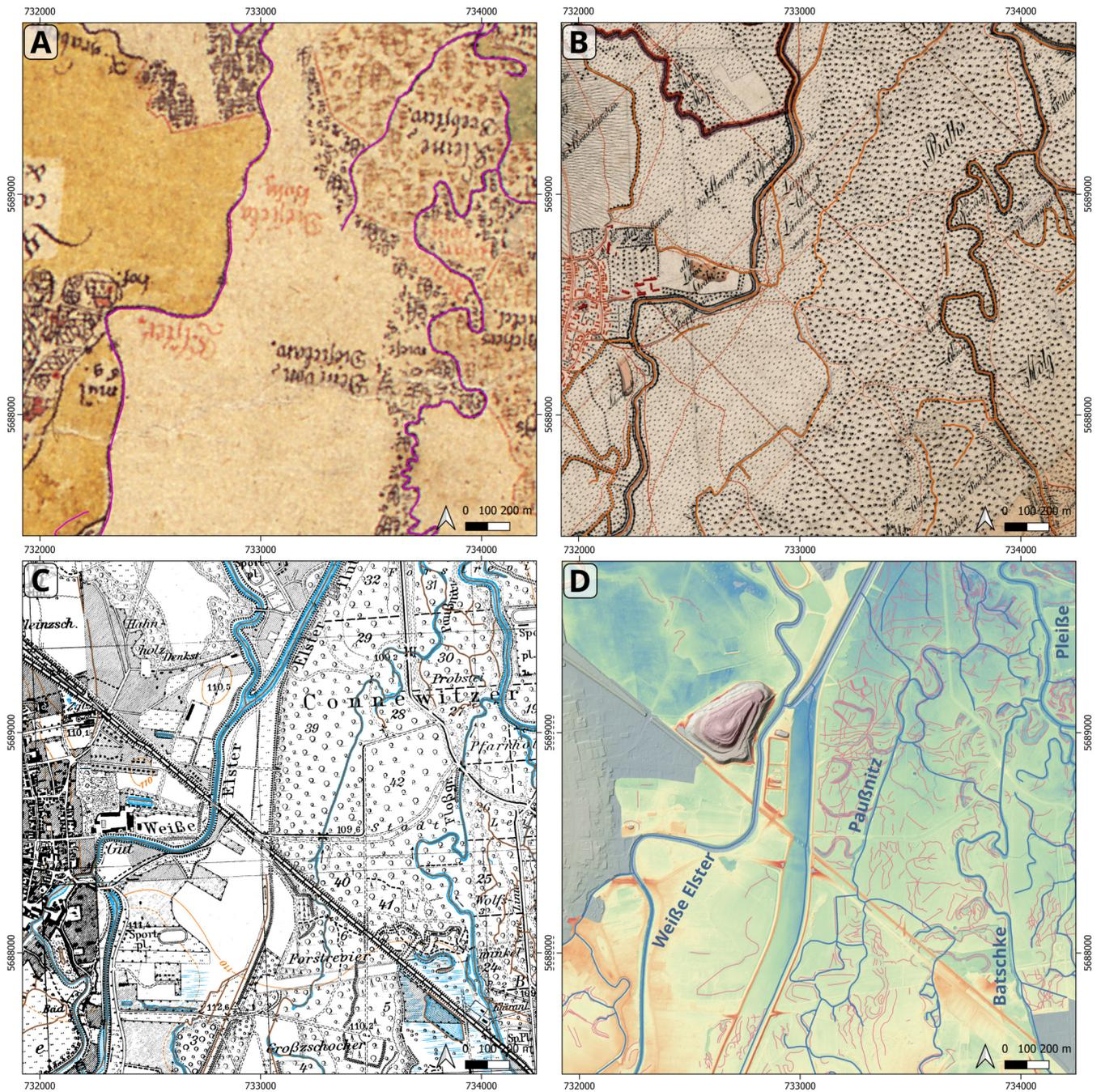
**Figure 3.** Sections of the study area with georeferenced old maps and the LiDAR DEM (Tab. 1 with vectorized rivers and channels (Tab. 2. A) Öder-Zimmermann (1585-1633 AD); B) *Meilenblätter von Sachsen, Berliner Exemplar* (1802 AD); C) *Messischblätter* (1930 AD); LiDAR DEM with mapped fluvial geomorphologic structures. EPSG:25832
