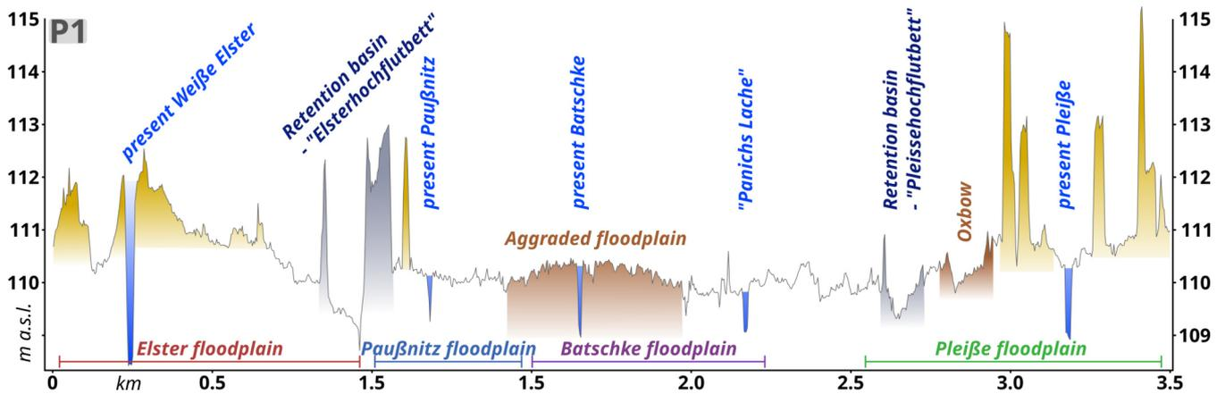
**Figure 5.** Topographic profile of the cross-section before the confluence of the tributaries based on the 1x1 m LiDAR DTM (GeoSN, 2018). The yellow color indicates modern infrastructure that alter the topography. The brown color highlights notable geomorphic features mentioned in the text. The location of the cross-section P1 is shown in Fig. 4A.
