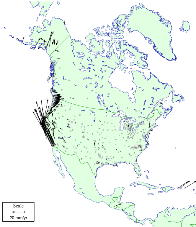
Figure 7: NAREF horizontal velocities after removal of NNR-NUVEL-1A model influence. Internal deformation is clearly visible, undermining assumptions of rigid plate behavior. From [6].
