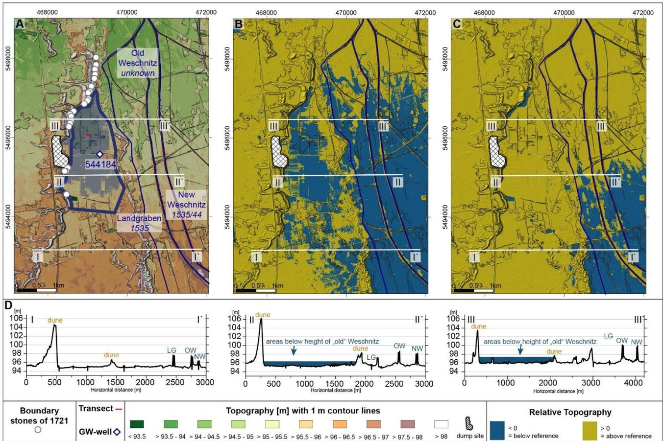
**Figure 3:** A) DGM1 with 1m contour lines for the Lake Lorsch area, mapping of boundary stones from 1721 (based on Schenk, 2024) and maximal extent for the lake (solid blue line) within the 94.5 to 95.5 m. a.s.l. height level (semi-transparent blue area); B) REM related to the course of the old Weschnitz; C) REM related to the course of the new Weschnitz; D) Topographical cross-sections in the southern, non-lake area (I-I'), middle lake area (II-II') and northern lake area (III-III').
