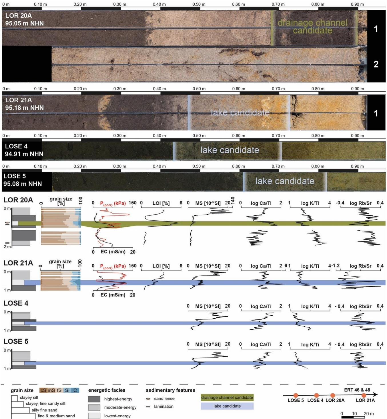
**Figure 7: Stratigraphy of sediment master cores LOR 20A and LOR 21A with results from Direct push hydraulic profiling (DP-HPT) and laboratory analyses (grain-size distribution, log, MS, log Ca/Ti, Log K/Ti and Log Rb/Sr) and short-cores LOSE 4 and LOSE 5.**
