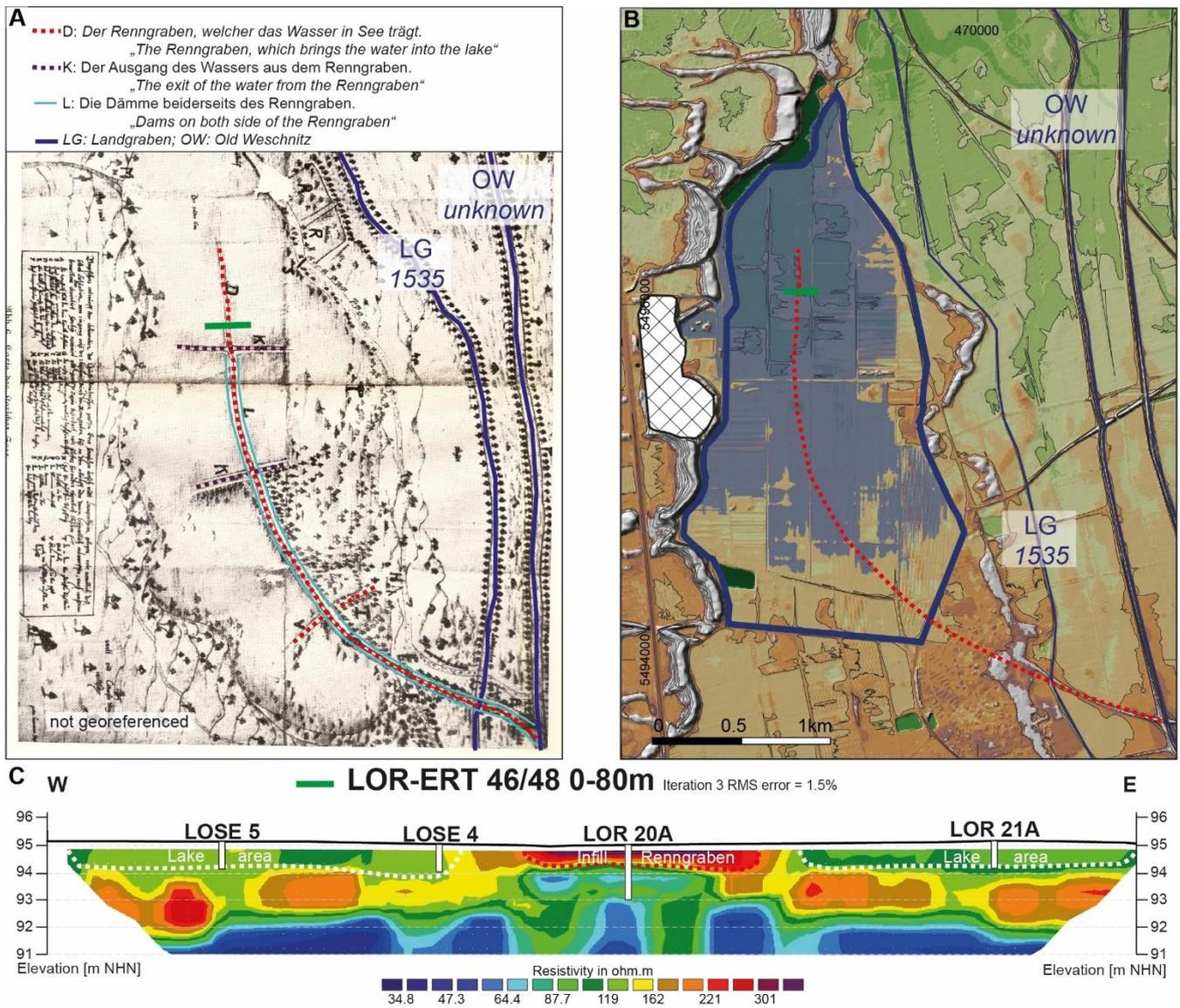
**Figure 6:** A) Lake Lorsch on an old map from 1700 (from Lepper, 1938) with emphasis on artificial channel (Renngraben) for water input at Lake Lorsch in comparison with B) digital elevation model (for Legend see figure 3) with location of postulated course of the Renngraben. C) ERT-transect ERT 46/48 with location of sediment cores.
