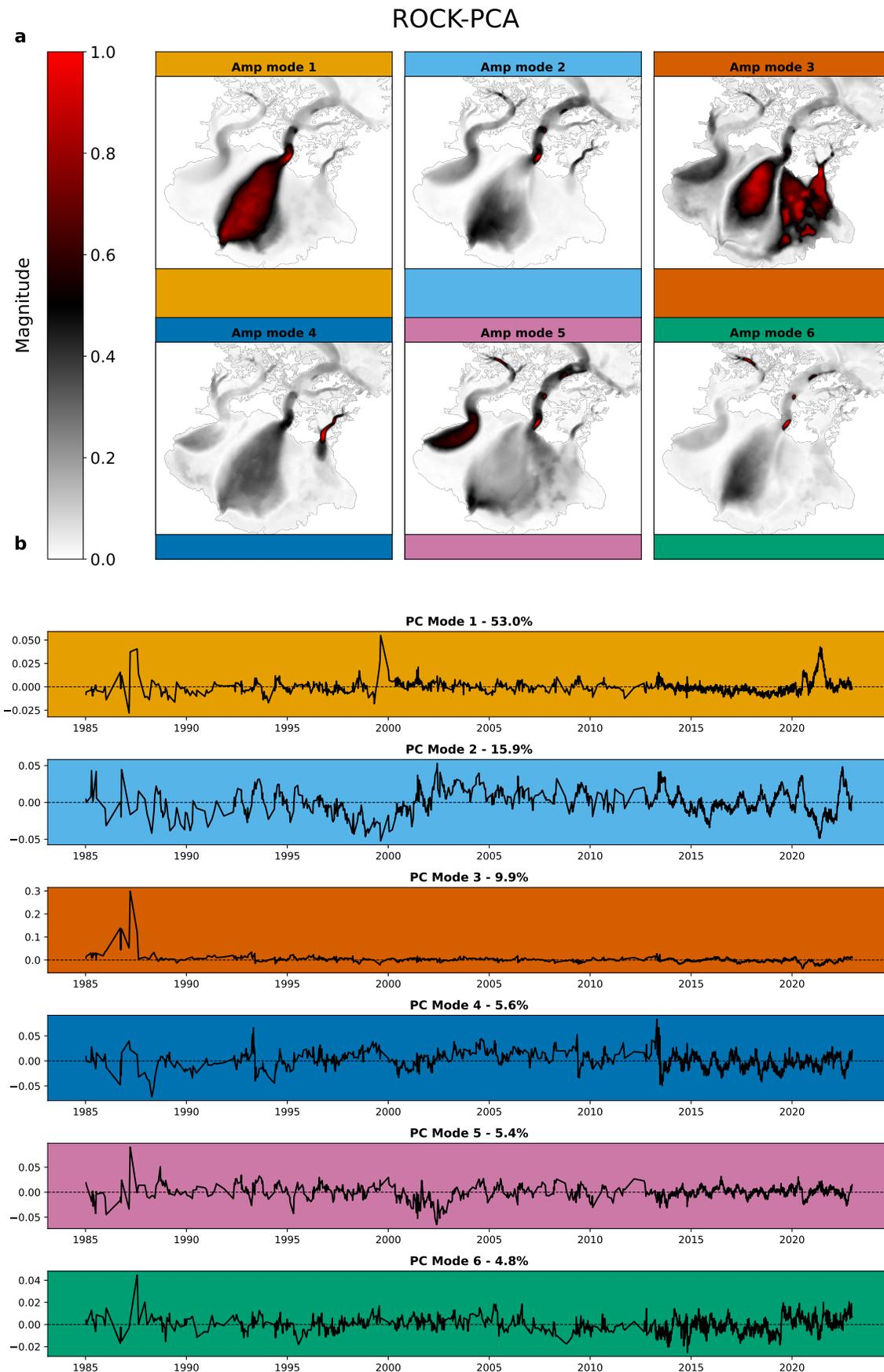
**Fig. 3.** a) Amplitude of the first 6 modes of the velocity. A non-zero amplitude represents changes in the variance. b) Principal Components (modes in times) with explained variance of the dataset (in %) associated to their respective modes (color coded). High positive values mean the spatial pattern is shown in (a) is at its maximum contrast. Negative values mean the spatial pattern is the opposite of the positive spatial pattern. Values around zero indicate that the spatial pattern is flat.
