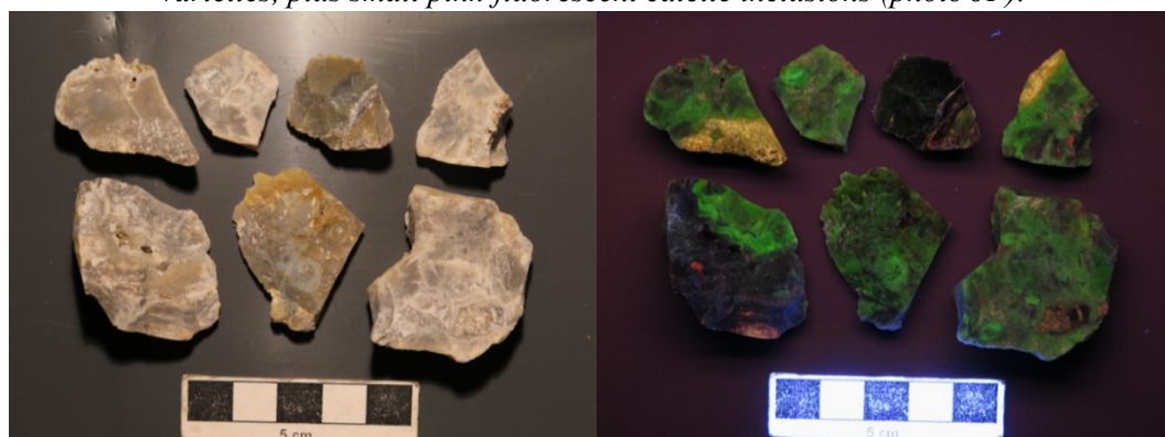
Fig. 6. (below) Randomly broken fragments, showing good flaking behaviour, from pebbles and boulders on Stotfield beach, Lossiemouth, showing green-, cream- and non-fluorescent chert varieties, plus small pink-fluorescent calcite inclusions (photo JF).
