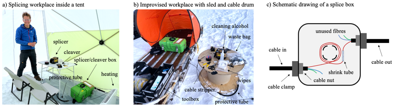
Figure 3. Optical fibre splicing in practice. a) Splicing workplace set up in a tent near the EastGRIP camp site on the Northeast Greenland Ice Stream. Ideally, splicing should be done by a team of two in an environment that allows for focused work for potentially several hours. b) An improvised workplace setup on a sled and a cable drum at several kilometres distance from the EastGRIP camp. c) Schematic drawing of a splice box. An important feature that not all commercially available boxes have are the cable clamps that offer some tensile strength, which is important in the field.
