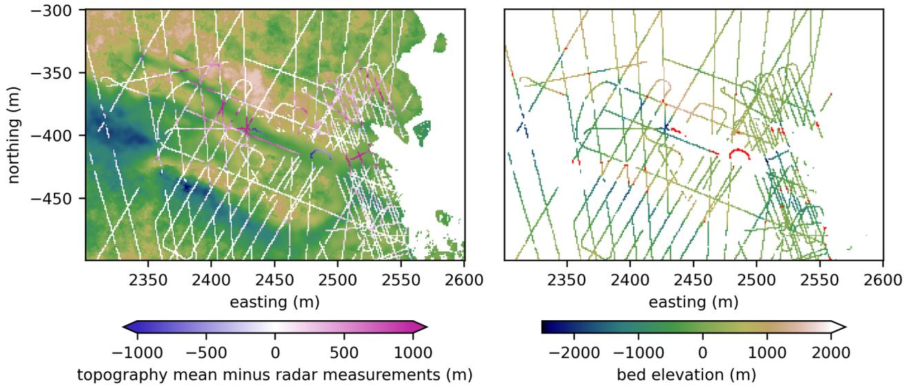
Figure S1: Subplot (a) shows the elevation differences between topography from the preprocessing chain and the radar-measured topography, which is overlaid upon the end topography sample generated in the preprocessing chain. Subplot (b) shows the radar-measured topography and the excluded bed elevation measurements highlighted in red
