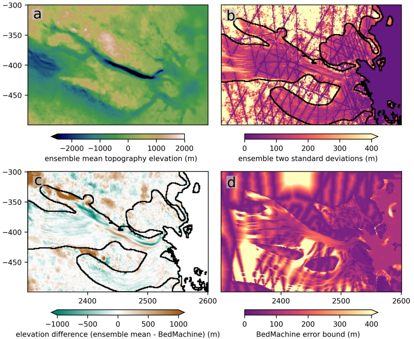
**Fig. 9.** (a) the ensemble mean bed elevation (m); (b) the ensemble standard deviation multiplied by two (m); (c) the elevation difference (ensemble mean - BedMachine; m); (d) the error bound of the BedMachine topography. The black outlines in (b) and (c) denote the high-velocity region, where the MCMC algorithm is applied
