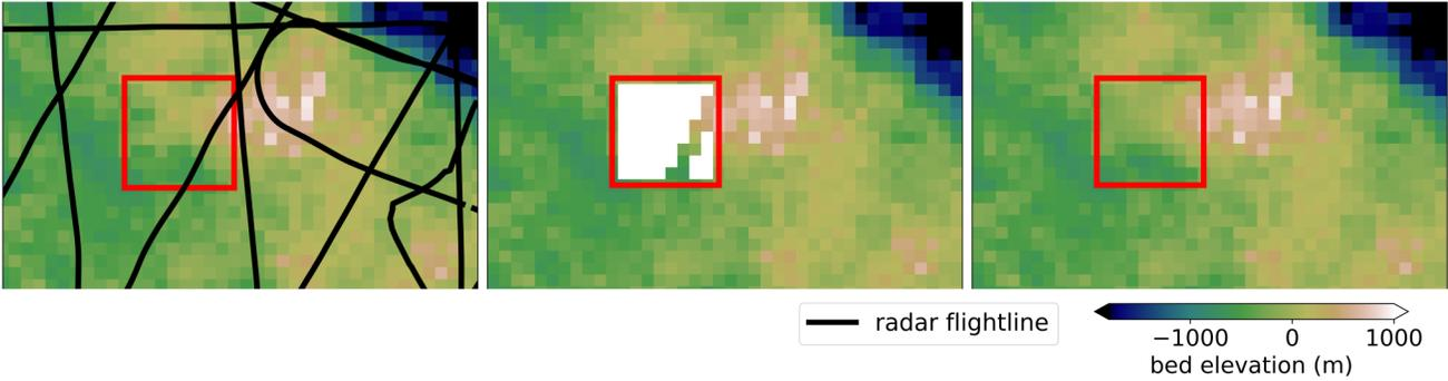
**Fig. 5.** An illustration of the update method used in the fine-scale chain. The red rectangle represents the selected random block.
