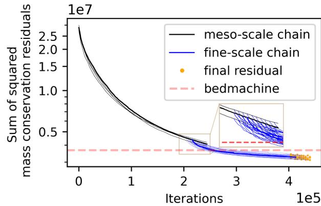
**Fig. 7.** The sum of squares of mass conservation residuals in the 4 meso-scale chains and the corresponding 40 fine-scale chains. The bold lines show an example of meso-scale chains and an example of fine-scale chains. The orange dots at the end of the lines denote the end sum of squared residuals of each topography realizations in the ensemble. The transition between meso-scale chains and fine-scale chains is enlarged in the inset figure.
