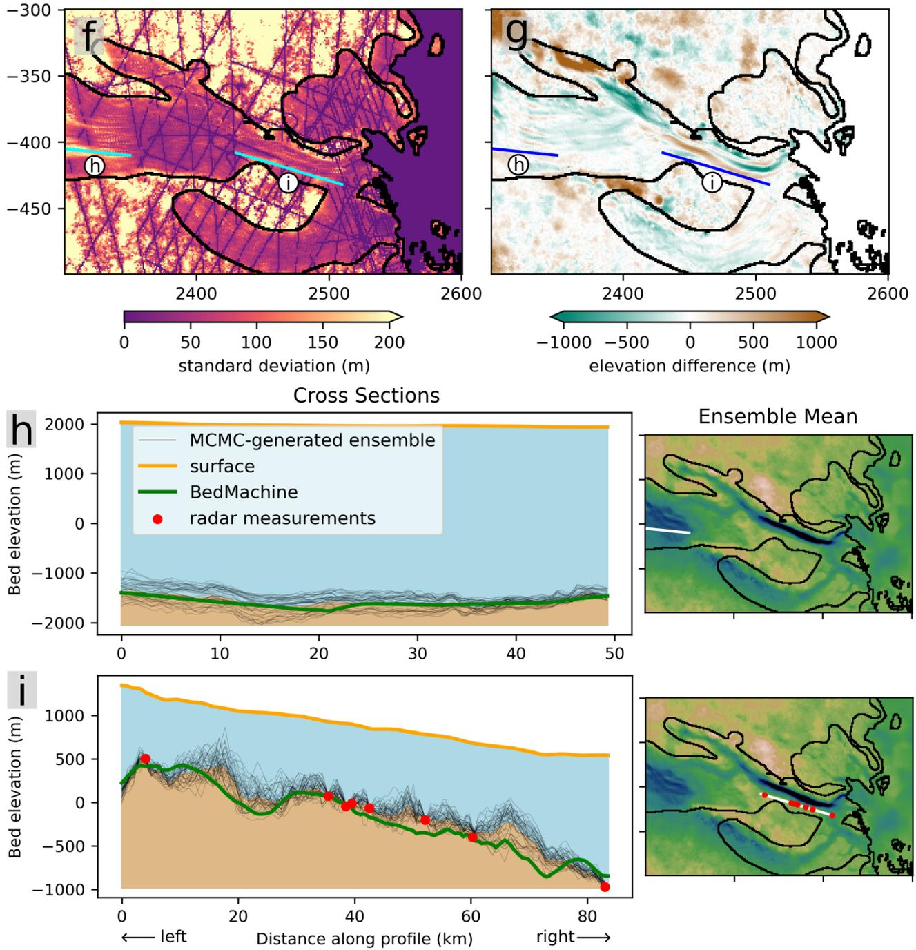
**Fig. 11.** Cross sections of the topography ensemble, where the transect lines go through two locations with high standard deviations. The layout and notations are similar to Fig. 10.
