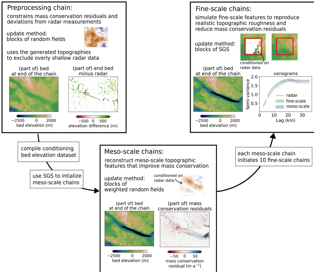
**Fig. 2.** Schematic overview of the workflow of the three MCMC chains.
