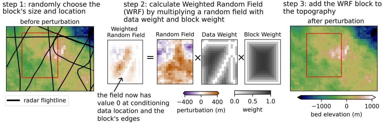
**Fig. 4.** An illustration of the update method used in the meso-scale chain. The red rectangle in step 1 and step 3 represent the selected random block.
