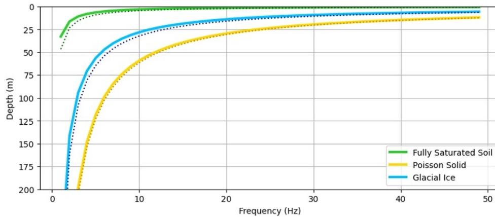
Frequency-dependent depths at which Rayleigh-wave particle motion change from retrograde to prograde for a fully saturated soil profile (green) (Yang, 2005), a Poisson's solid (yellow) (Ammon and others, 2020), and glacial ice (blue) based on parameters estimated for the Saskatchewan Glacier (Stevens and others, 2023). Solid lines are analytical solutions (Eqn. (5)), and dotted lines are approximated depths (Eqn. (6)) for all models. Table 1 lists associated material properties.
