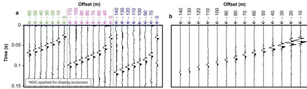
(a) Time-aligned Z-component shot gathers for stations S02 (blue), S05 (pink), and S09 (green) with differing offset ranges (x-axis labels). (b) Supergather produced from stacking the three shots in (a) based on similar offsets thus increasing the effective array aperture to  $L=130$  m and infilling missing offset traces without interpolation.
