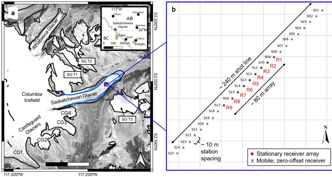
**Fig. 16.** (a) Saskatchewan Glacier location in the Canadian Rocky Mountains, Canada (see inset map). Basemap imagery: Orthorectified 4-band PlanetScope scene accessed via Planet.com (b) Geometry of the active-source seismic experiment conducted in the ablation zone involving a stationary array of nine 3-C geophones (R1-R9) linearly spaced at 10 m to form an array of aperture  $L = 80$  m. Source station locations S01-S25, also spaced 10 m apart, are shown as blue Xs.
