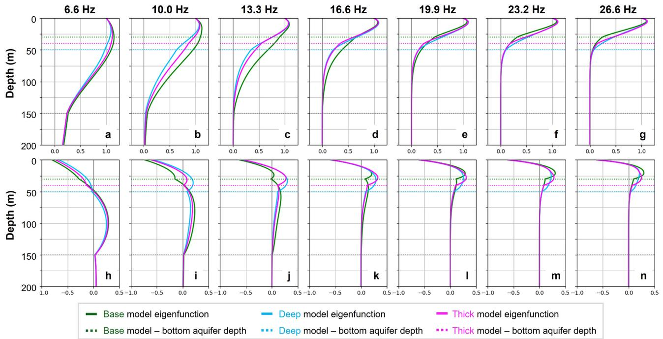
**Fig. 15.** Depth sensitivity kernels for discrete frequencies of the three aquifer-firn experiments described in Fig. 12. (a–g)  $U_z$  components. (h–n)  $U_x$  components. Depths of the bottom of aquifer are color coded for each model, and the depth of the ice-bedrock interface is shown with a dotted gray line at 150 m. The unique sensitivities of the  $U_x$  curves for each model motivate an opportunity for improving MASW inversion accuracy through use of MC data.
