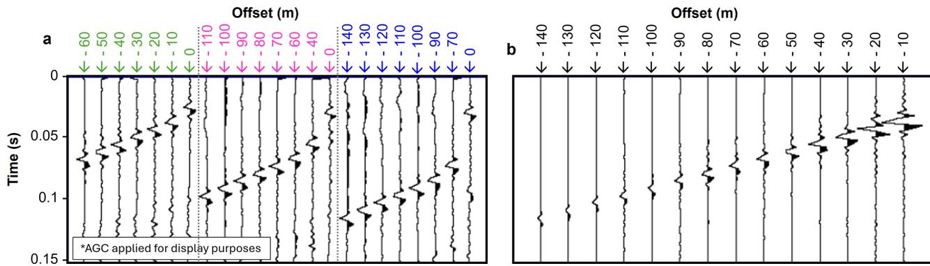
**Fig. 19.** (a) Time-aligned Z-component shot gathers for stations S02 (blue), S05 (pink), and S09 (green) with differing offset ranges ( $x$ -axis labels). (b) Supergather produced from stacking the three shots in (a) based on similar offsets thus increasing the effective array aperture to  $L = 130$  m and infilling missing offset traces without interpolation.
