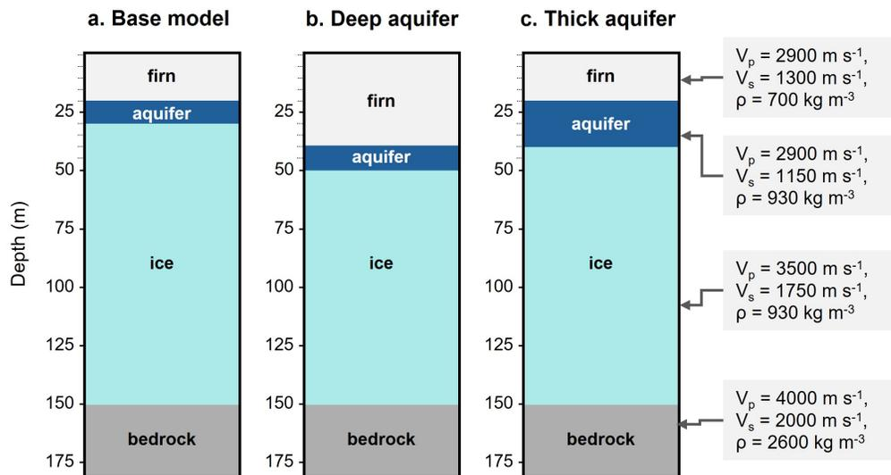
**Fig. 12.** Firm-aquifer model variations for synthetic data generation. (a) “Base” model derived from Helheim Glacier seismic inversion results (Killingbeck and others, 2018) with a 10 m thick aquifer overlain by 20 m of firn and a bedrock half-space imposed at 150 m depth. (b) “Deep Aquifer” model similar to (a) but with the firn layer extended to a depth of 40 m. (c) “Thick Aquifer” model similar to (a) but with the aquifer thickened to 20 m.
