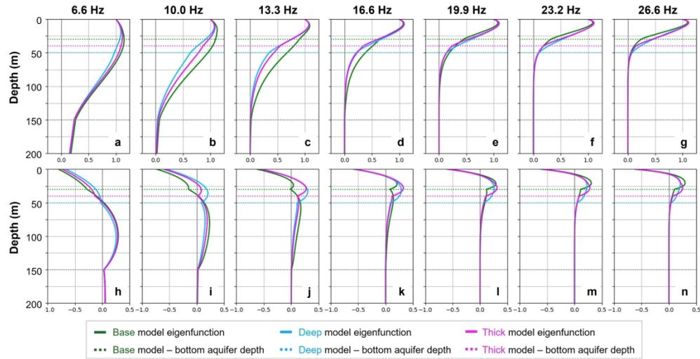
Depth sensitivity kernels for discrete frequencies of the three aquifer-firn experiments described in Fig. 12. (a--g)  $U_z$  components. (h--n)  $U_x$  components. Depths of the bottom of aquifer are color coded for each model, and the depth of the ice-bedrock interface is shown with a dotted gray line at 150 m. The unique sensitivities of the  $U_x$  curves for each model motivate an opportunity for improving MASW inversion accuracy through use of MC data.
