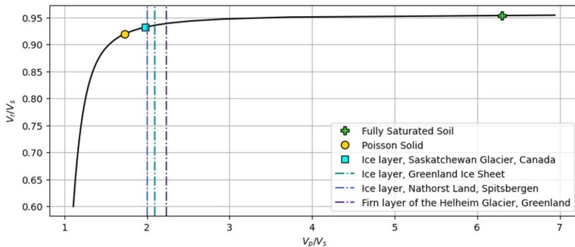
**Fig. 4.** Rayleigh-wave characteristic equation (Eqn. (7)) represented as a relationship between  $V_p/V_s$  and  $V_r/V_s$  (black curve) with reference values for a saturated soil (green cross), Poisson solid (yellow circle), and glacial ice at the Saskatchewan Glacier (cyan square).  $V_p/V_s$  estimates of other glacial examples are plotted as vertical lines since  $V_r/V_s$  estimates are not mentioned in reference studies. Table 1 lists associated material properties.
