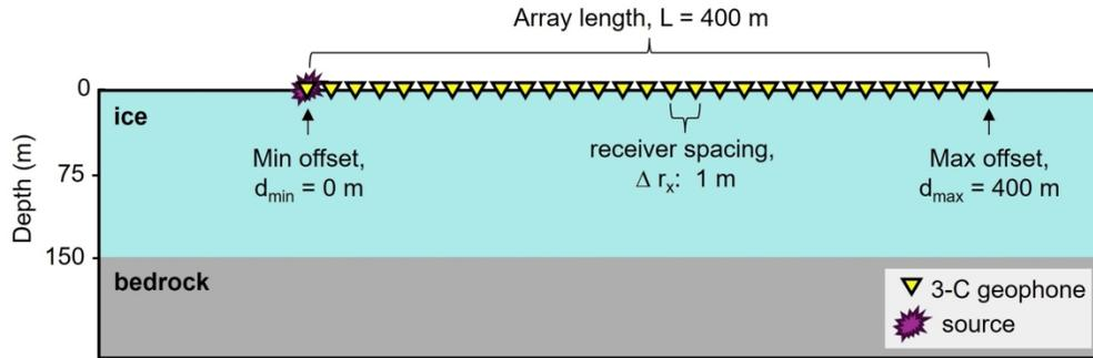
Model describing a homogeneous, isotropic, elastic ice layer of 150 m thickness overlying a bedrock half space. Table 2 presents the elastic model properties. The idealized acquisition has a dense 1 m receiver spacing and 400 m aperture. The sketched geometry is not to scale and approximates receiver placement for visual reference.
