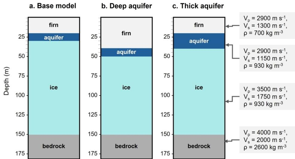
Firn-aquifer model variations for synthetic data generation. (a) "Base" model derived from Helheim Glacier seismic inversion results (Killingbeck and others, 2018) with a 10 m thick aquifer overlain by 20 m of firn and a bedrock half-space imposed at 150 m depth. (b) "Deep Aquifer" model similar to (a) but with the firn layer extended to a depth of 40 m. (c) "Thick Aquifer" model similar to (a) but with the aquifer thickened to 20 m.
