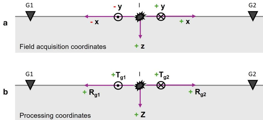
**Fig. 1.** Definition of the (a) acquisition coordinate system in horizontal  $x$  and  $y$  and vertical  $z$  directions, and (b) the cylindrical processing coordinate system in outward-positive radial  $R$  and vertical  $Z$  directions. The transverse,  $T$  direction is always counter clockwise from  $R$ .  $I$  and  $G$  annotate the locations of the impact source and receivers in each sketch.
