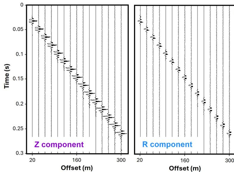
**Fig. 13.** Conditioned  $Z$ - and  $R$ -component shot gathers for the “base” firn-aquifer model described in Fig. 12. Every 20th trace is plotted for offsets ranging from 20 m to 300 m.
