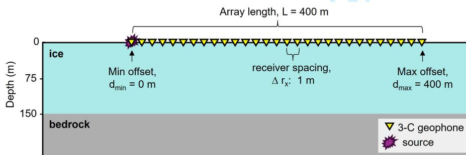
**Fig. 5.** Model describing a homogeneous, isotropic, elastic ice layer of 150 m thickness overlying a bedrock half space. Table 2 presents the elastic model properties. The idealized acquisition has a dense 1 m receiver spacing and 400 m aperture. The sketched geometry is not to scale and approximates receiver placement for visual reference.
