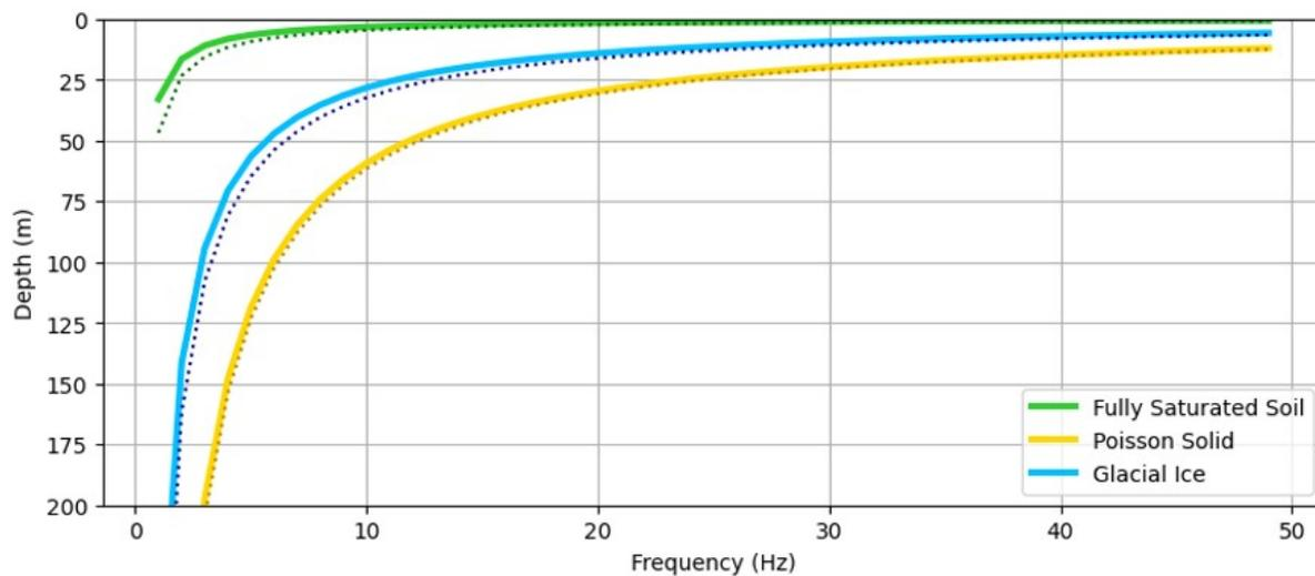
**Fig. 3.** Frequency-dependent depths at which Rayleigh-wave particle motion change from retrograde to prograde for a fully saturated soil profile (green) (Yang, 2005), a Poisson's solid (yellow) (Ammon and others, 2020), and glacial ice (blue) based on parameters estimated for the Saskatchewan Glacier (Stevens and others, 2023). Solid lines are analytical solutions (Eqn. (5)), and dotted lines are approximated depths (Eqn. (6)) for all models. Table 1 lists associated material properties.
