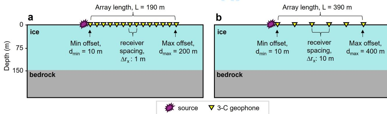
**Fig. 10.** Two-layer ice-bedrock model described in Table 2 with two different acquisition experiments: (a) an aperture of  $L = 190$  m (approximately half the length of the example described in Fig. 5) and a receiver spacing of  $\Delta r_x = 1$  m with the zero-offset receiver removed; and (b) an aperture of  $L = 390$  m and a receiver spacing of  $\Delta r_x = 10$  m. Not drawn to scale with the receiver placement only approximate for visual reference.
