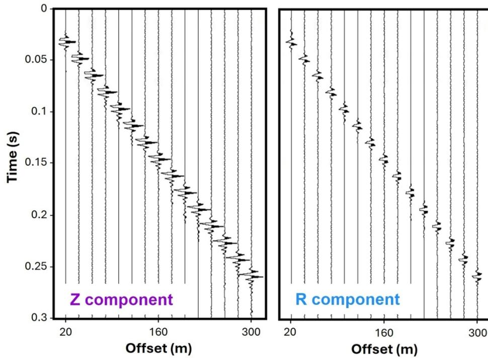
Conditioned Z- and R-component shot gathers for the ``base'' firn-aquifer model described in Fig. 12. Every 20th trace is plotted for offsets ranging from 20 m to 300 m.
