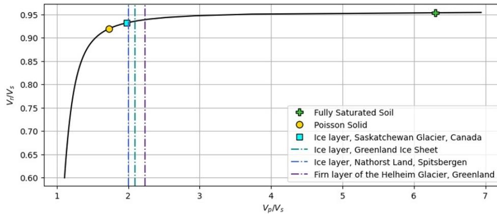
Rayleigh-wave characteristic equation (Eqn. (7)) represented as a relationship between  $V_p/V_s$  and  $V_r/V_s$  (black curve) with reference values for a saturated soil (green cross), Poisson solid (yellow circle), and glacial ice at the Saskatchewan Glacier (cyan square).  $V_p/V_s$  estimates of other glacial examples are plotted as vertical lines since  $V_r/V_s$  estimates are not mentioned in reference studies. Table 1 lists associated material properties.
