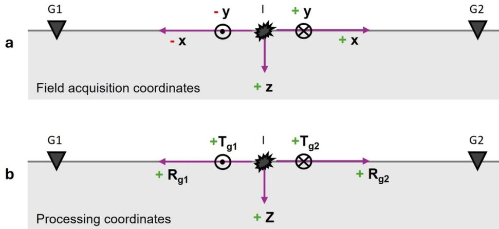
Definition of the (a) acquisition coordinate system in horizontal ( $x$  and  $y$ ) and vertical ( $z$ ) directions, and (b) the cylindrical processing coordinate system in outward-positive radial  $R$  and vertical  $Z$  directions. The transverse,  $T$  direction is always counter clockwise from  $R$ .  $I$  and  $G$  annotate the locations of the impact source and receivers in each sketch.
