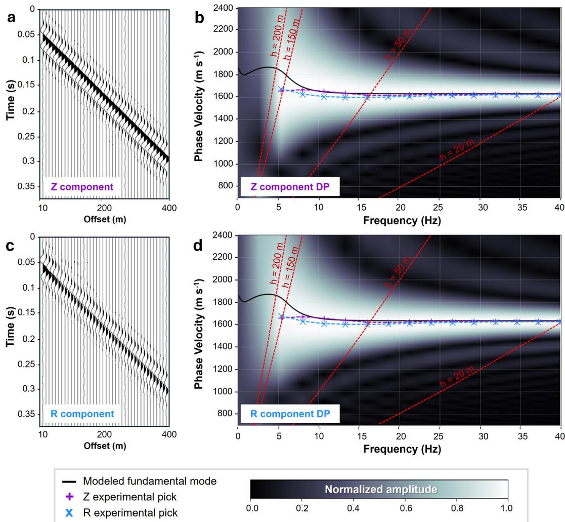
**Fig. 9.** Conditioned shot gather data and DPs after removing the direct P-wave arrival and windowing out noisy near-offset traces to highlight the full Rayleigh-wave character at far offsets. See Fig. 6 for descriptions of individual panels. We improved sub-10 Hz resolution of the DPs with appropriate data conditioning.
