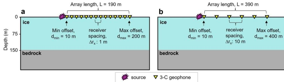
Two-layer ice-bedrock model described in Table 2 with two different acquisition experiments: (a) an aperture of  $L=190$  m (approximately half the length of the example described in Fig. 5) and a receiver spacing of  $\Delta r_x=1$  m with the zero-offset receiver removed; and (b) an aperture of  $L=390$  m and a receiver spacing of  $\Delta r_x=10$  m. Not drawn to scale with the receiver placement only approximate for visual reference.
