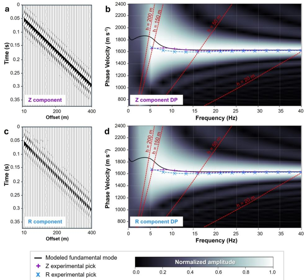
Conditioned shot gather data and DPs after removing the direct P-wave arrival and windowing out noisy near-offset traces to highlight the full Rayleigh-wave character at far offsets. See Fig. 6 for descriptions of individual panels. We improved sub-10 Hz resolution of the DPs with appropriate data conditioning.
