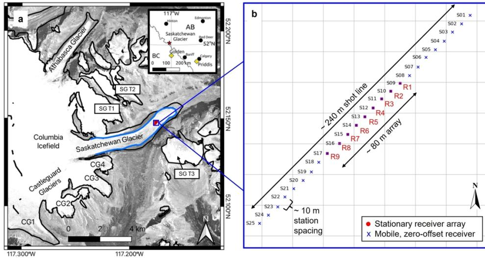
(a) Saskatchewan Glacier location in the Canadian Rocky Mountains, Canada (see inset map). Basemap imagery: Orthorectified 4-band PlanetScope scene accessed via Planet.com (b) Geometry of the active-source seismic experiment conducted in the ablation zone involving a stationary array of nine 3-C geophones (R1-R9) linearly spaced at 10 m to form an array of aperture  $L=80$  m. Source station locations S01-S25, also spaced 10 m apart, are shown as blue Xs.
