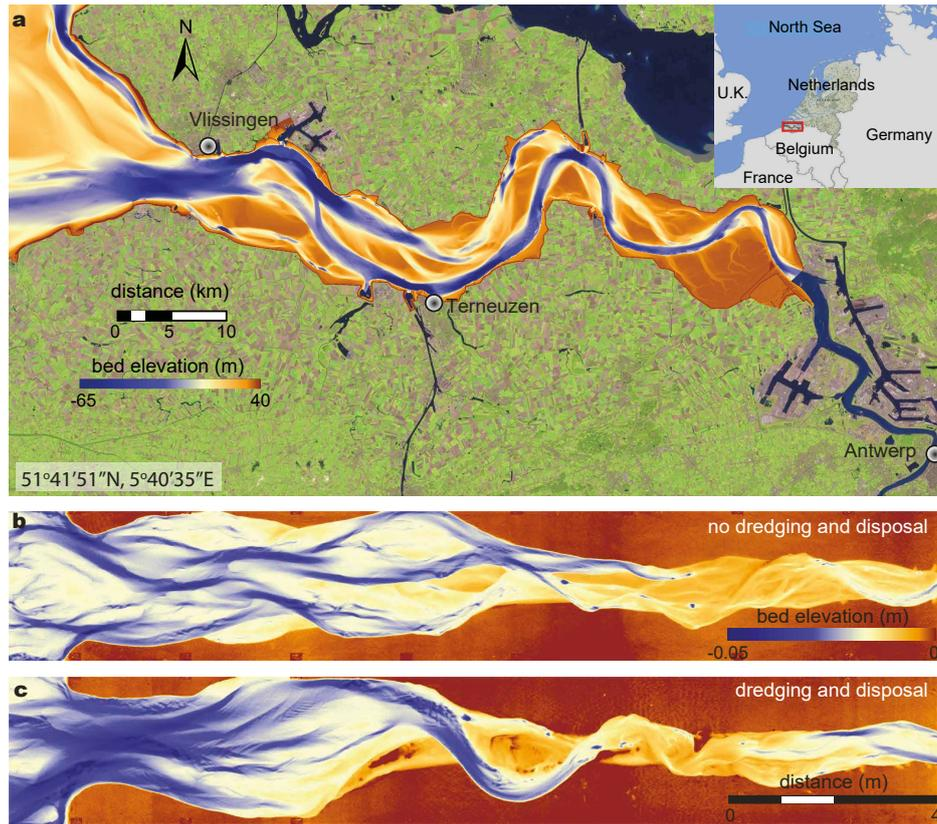
**Figure 1.** Bed elevation maps for the Western Scheldt and two flume experiments. a) 2014 bed elevation of the Western Scheldt. b) Final bed elevation for the control run after 13,000 tidal cycles. c) Final bed elevation after 13,000 tidal cycles for the experiment with dredging and disposal (DaD) occurring between 3,000-5,200 tidal cycles.
