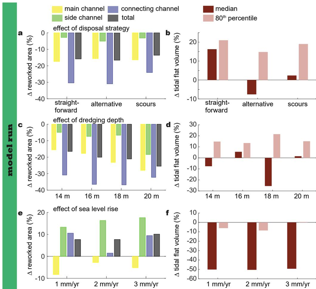
**Figure 4.** Effect of future scenarios on reworking by channels and tidal flat volume compared to the control run. a) Effect of disposal strategy on changes in the reworked area. b) Effect of disposal strategy on changes in tidal flat volume. c) Effect of dredging depth on changes in the reworked area. d) Effect of dredging depth on changes in tidal flat volume. e) Effect of sea-level rise on changes in the reworked area. f) Effect of sea-level rise on changes in tidal flat volume.
