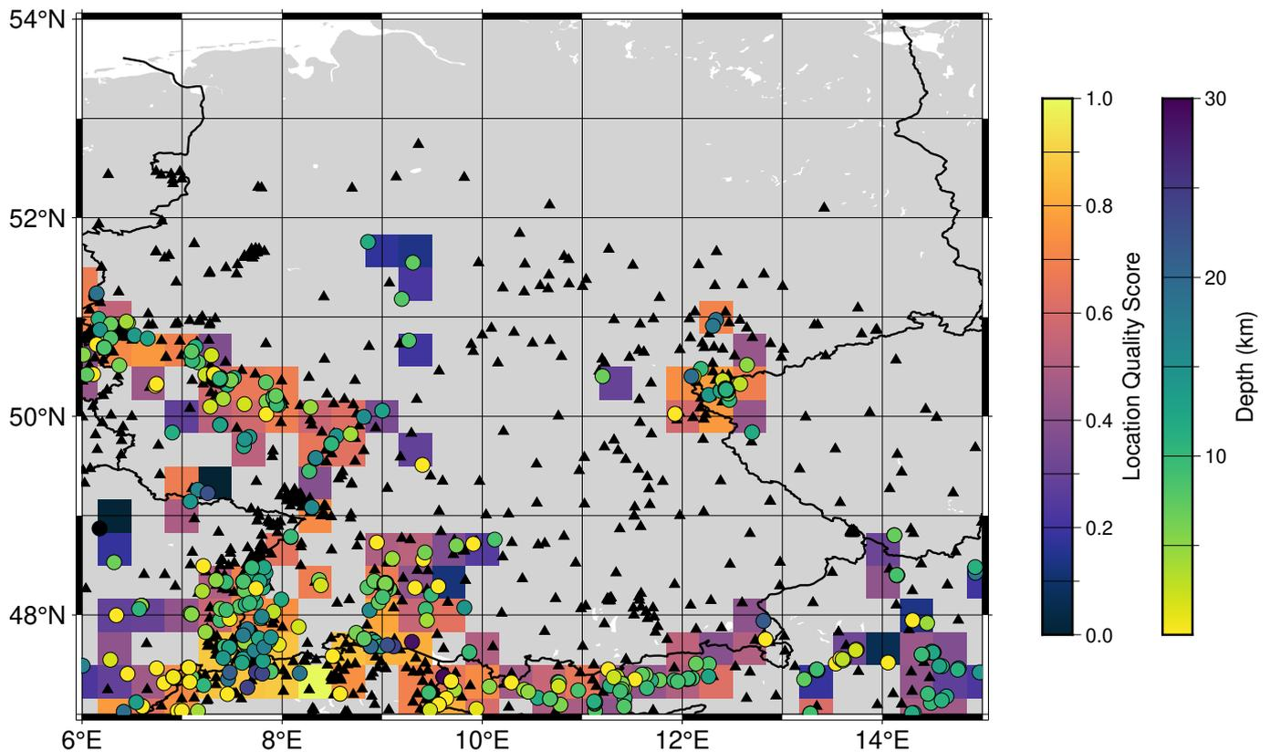
**Figure 4** Location Quality Score (LQS) for the 594 automatically located events, averaged within a  $20 \times 20$  m grid. Event locations are color-coded by automatically estimated depths (values clipped at 30 km). Black triangles denote seismic stations, including temporary deployments, used for phase picking during automatic location.
