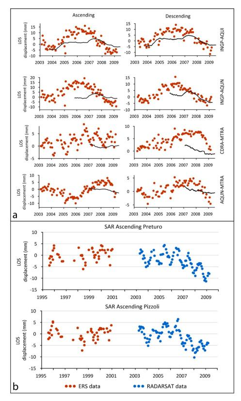
Figure 1: a) Differences between the displacements measured at some selected couples of GPS sites
