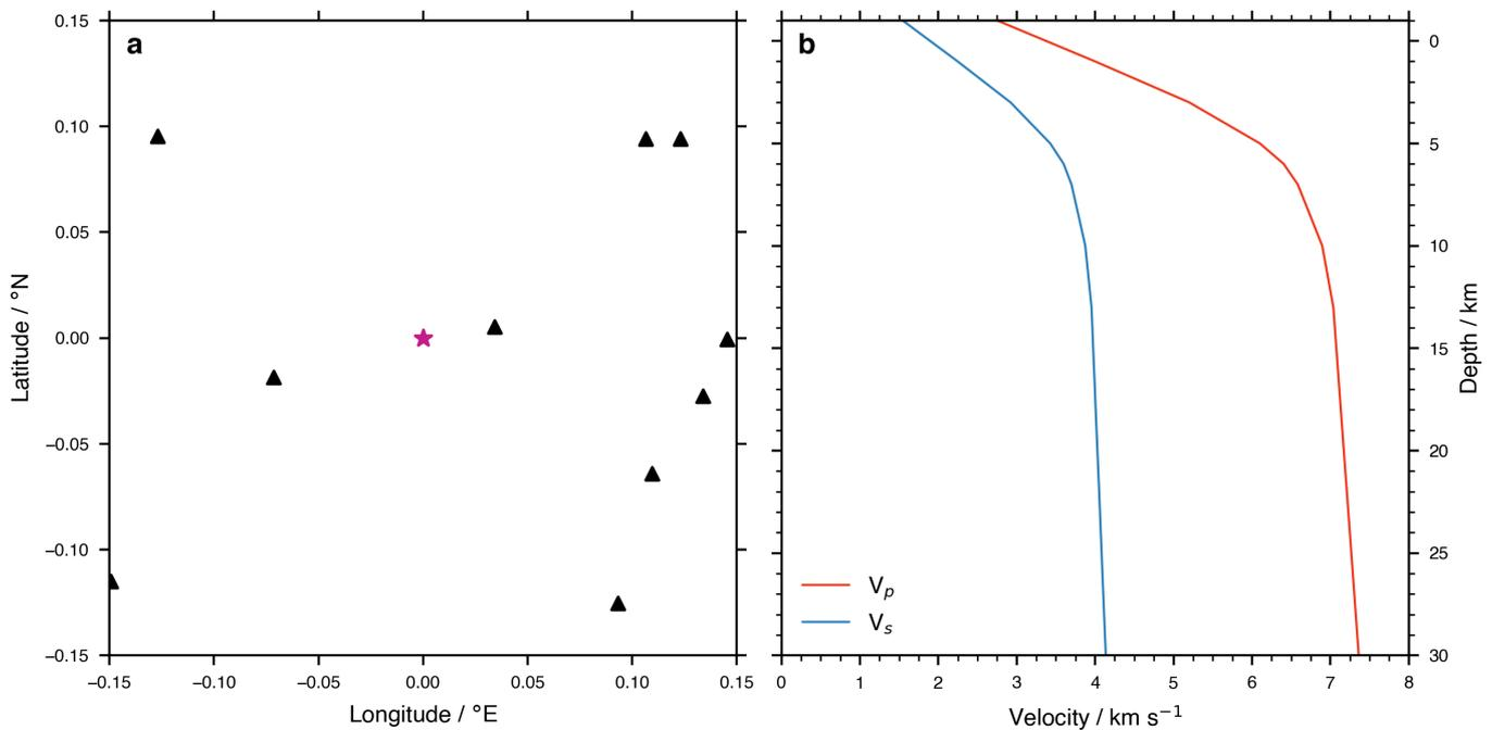
**Figure S1** Network geometry and velocity model for the synthetic test. a) Map view of the seismic network, with black triangles denoting the seismic stations, and the synthetic source denoted by the pink star. b) The 1-D P- and S-wave velocity model.
