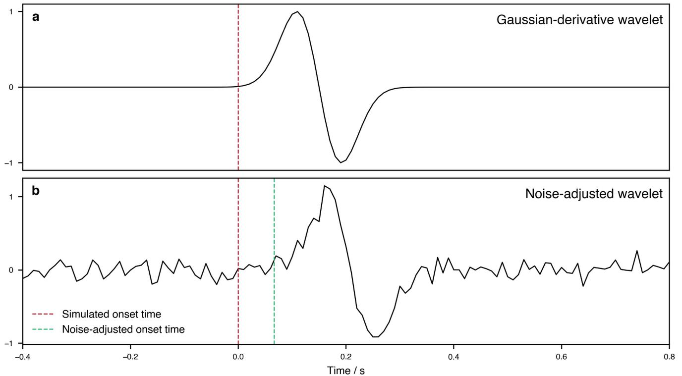
**Figure S2** Illustration of: a) the Gaussian-derivative wavelet and b) the effect of the synthetic noise added to the station-phase traveltimes and the waveform amplitudes.
