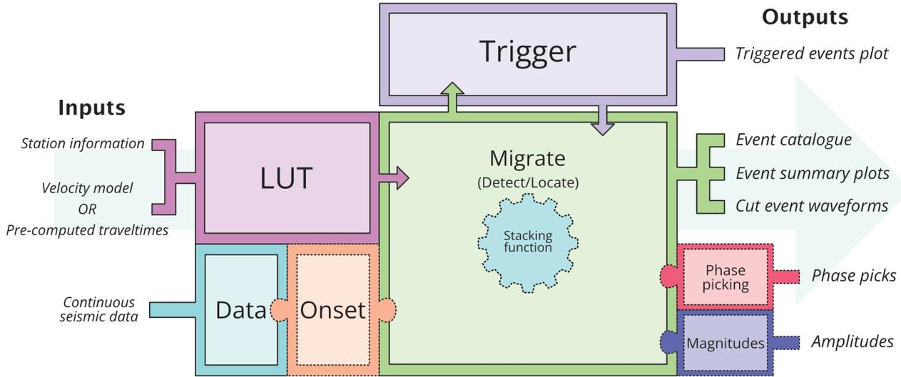
**Figure 2** Schematic illustrating the structure of the QuakeMigrate software package. Sections with dashed outlines (Onset, Pick and Magnitudes) are plugin/extension modules of the code that can be customised or substituted for alternatives by the user; arrows indicate the sequence of steps in the processing workflow.
