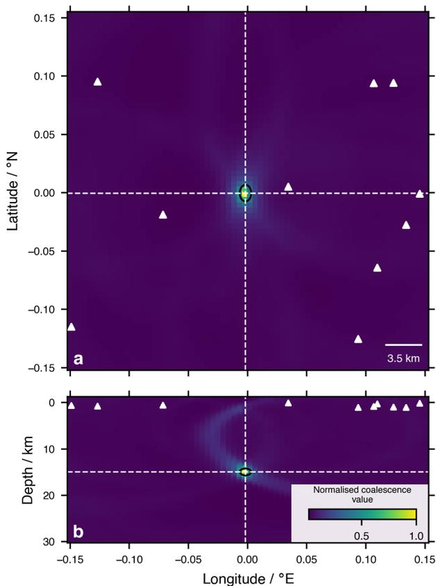
**Figure 5** QuakeMigrate event location plot for the synthetic example. a) shows a map view of a horizontal slice through the 3-D coalescence map at the earthquake hypocentre, coloured by normalised coalescence value. b) shows a longitude-depth cross-section. White dashed lines indicate the maximum probability location; black ellipse delineates a Gaussian estimate of the event location uncertainty.
