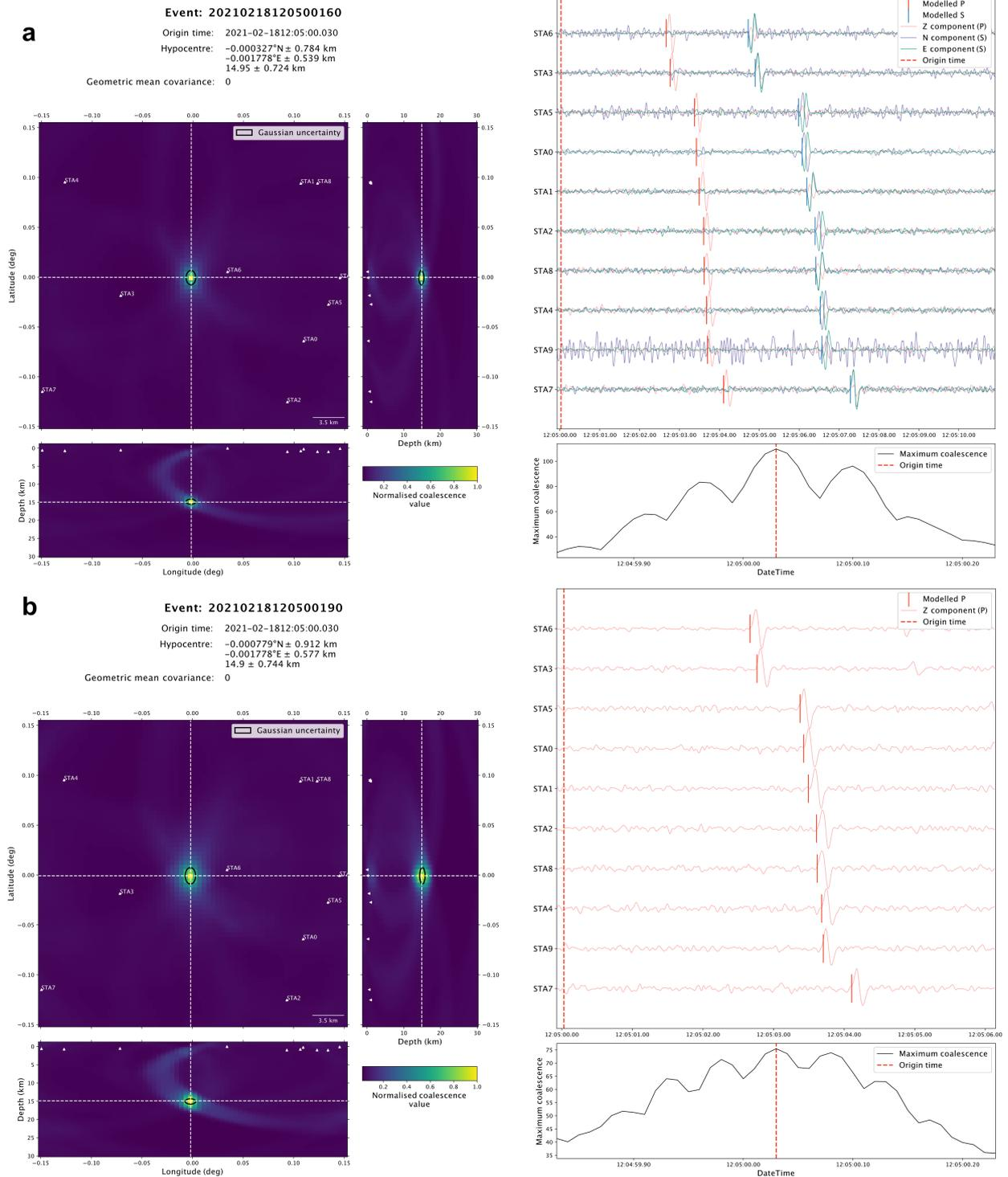
**Figure S3** Comparison of the locations derived from **a** using both the P- and S-phase arrivals and **b** using purely P-phase arrivals (i.e., only calculating, migrating, and stacking the P-onset function from the Z component). These are examples of the built-in event summary generated as part of the standard QuakeMigrate Locate function.
