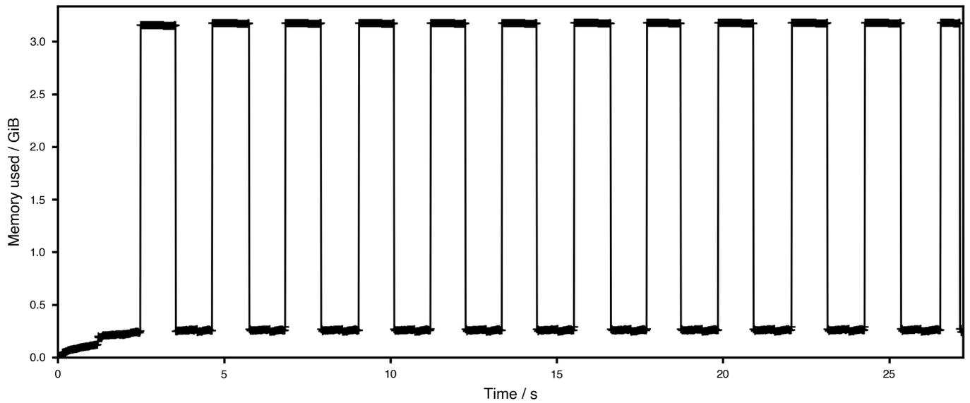
**Figure S6** Overview of the memory usage through time for the Detect stage. It can be seen that the program cycles between low memory usage (waveform pre-processing) and high memory usage (during the migration and stacking).
