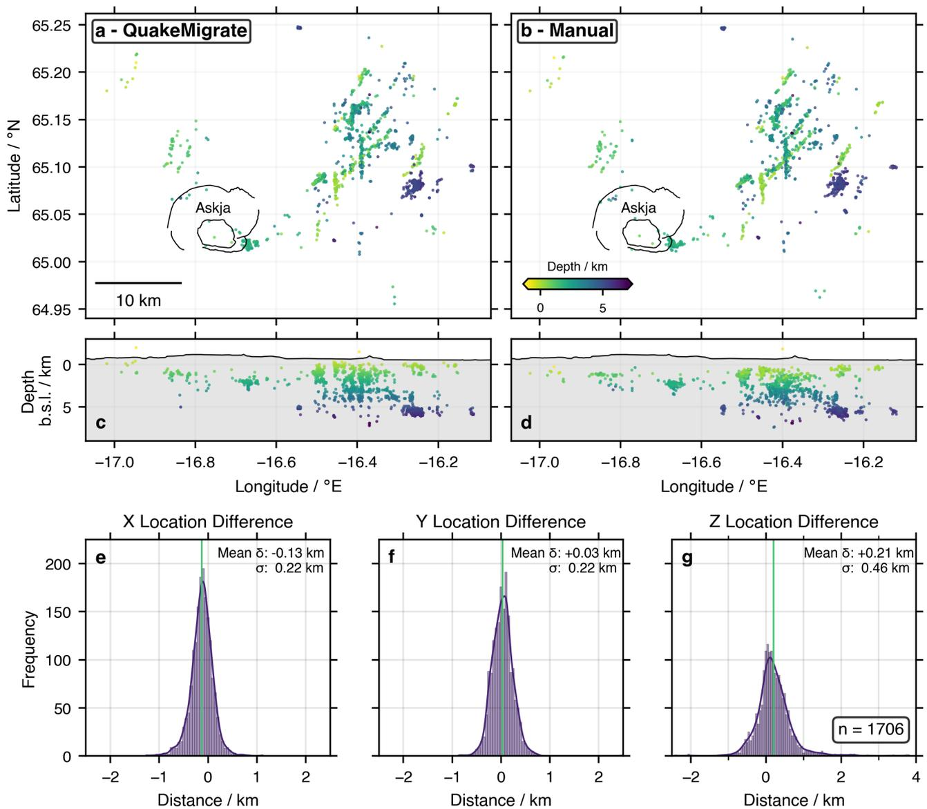
**Figure 10** Location comparison for manually analysed events around Askja between 2007–2015. **a** and **b** show map views for QuakeMigrate and NLLoc locations, respectively, with events coloured by depth; map area is the same displayed in Figure 9. **c** and **d** show cross-section views. **e**, **f** and **g** show location differences between QuakeMigrate and NLLoc locations across 1,706 events.
