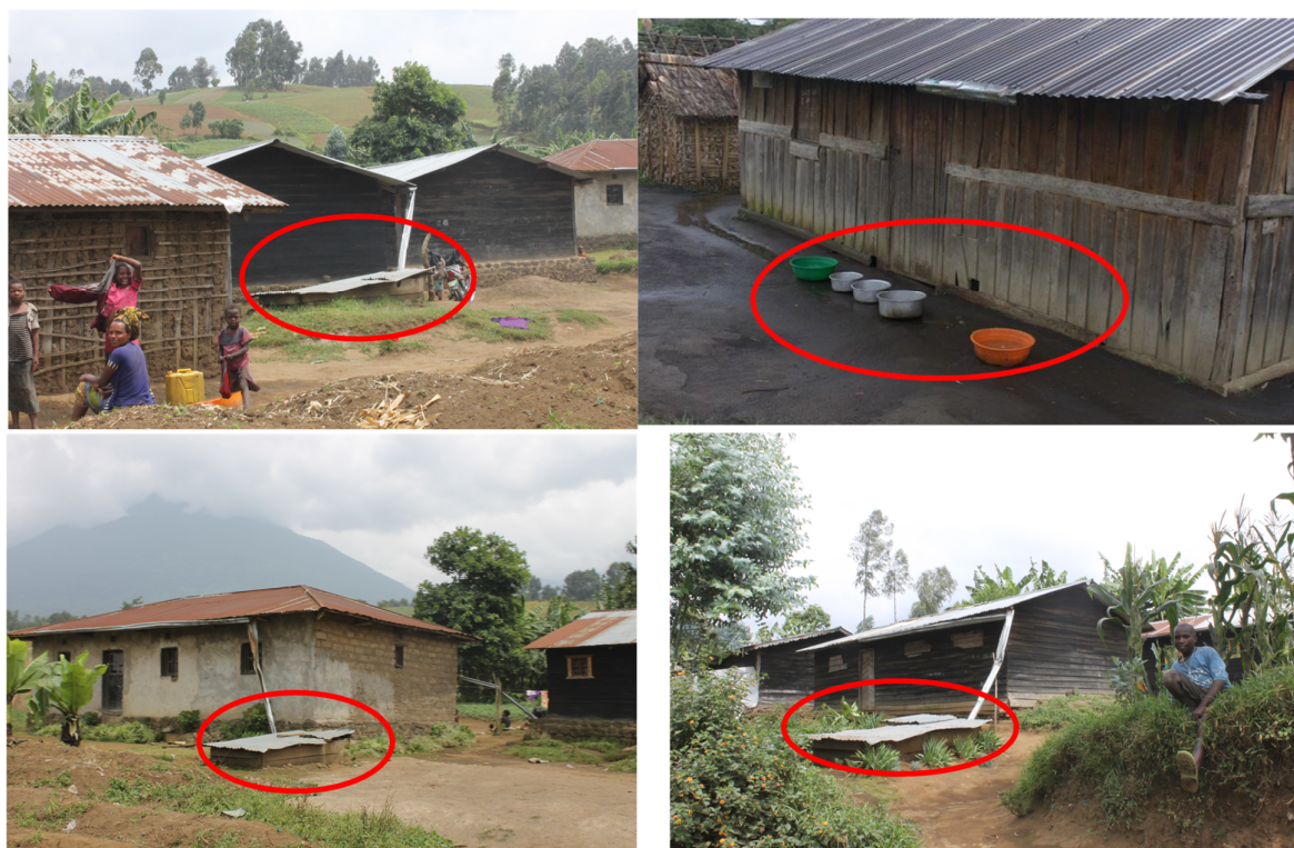
Figure 11. Photos showing the techniques of rainwater harvest in villages located around Nyiragongo and Nyamulagira volcanoes, and where the rainwater is the unique water source which is thus used for all daily activities, including for drinking.
